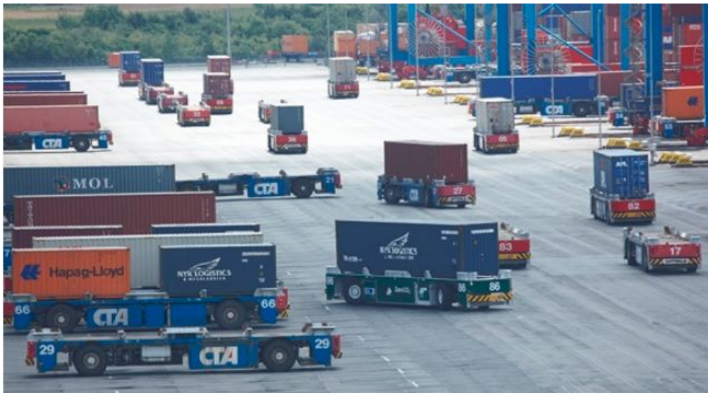
Figure 5. Automated guided vehicles (AGVs) are often utilized in ports for increasing productivity and efficiency
