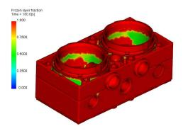
(a) Frozen layer fraction result. A complete view of the piece.
