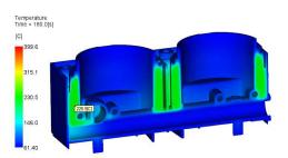
(b) Detail of the Temperature result of the complete analysis. The result is shown at 180 seconds of the cycle, in sectioned view, and one detailed point is chosen to be shown. For the point in the picture, the temperature is 226.5 C, clearly still above the transition temperature.
