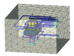
Figure 4.15: Mold mesh for Cool (BEM) analysis.
