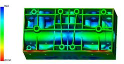
(b) Gate suitability. Back of the piece. The rib structure on the piece's rear part prevents having a good injection point on this side.
