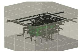
Figure 4.11: View of the mold block defined through the mold block wizard over the system with all the channels that could be imported and meshed up until this moment. The mesh of the mold was never achieved by the software.
