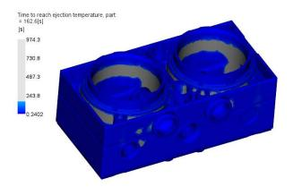
Figure 4.18: View of the part of the piece that is not frozen by the time set by the company, shown in grey. Most of the piece is not already frozen.
