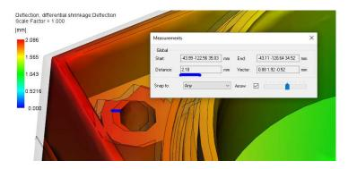
Figure A.6: Detail of the deflection for differential shrinkage.
