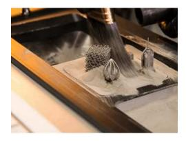
Figure 2.7: Product extraction of a DMLS process. Act of eliminating the excess powder to see the final product before detachment from the base. The complexity of the shapes that are possible to be obtained is clear in the image.
