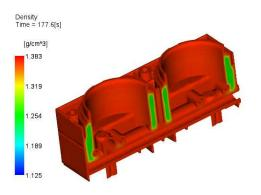
(a) Density of the material after the packing and cooling phase. Section view of the thickest point of the piece
