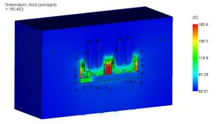
(c) Temperature of the mold, averaged. Section view of the point of maximum temperature
