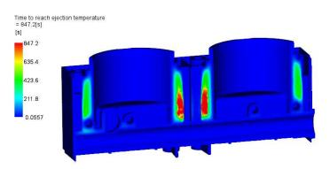
Figure A.8: Time to reach ejection temperature for the piece when the software is set for automatic time.
