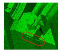
(b) Geometrical voids found in the structure. Their presence was spotted with the previously described gate analysis. The position of the best node for gate location is found here for this case.
