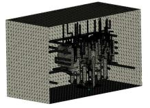
(d) Mold block section view when meshing the mold in second step - 3D mesh obtained
