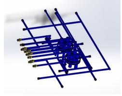
Figure 4.3: Cooling system on the fixed part of the mold. Solidworks file received from the company.
