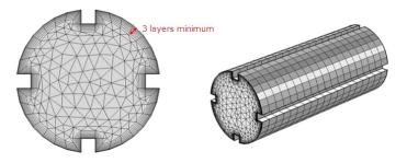
Figure 4.7: Enhancement layers required in any 3D cooling channel mesh. [34]
