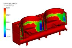
(b) Section view of the piece that shows how the injection area of the piece is still completely liquid by the end of the cycle time. This is the most critical point of the piece for this result.
