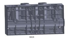
Figure 1.4: Perspective view of the back of the piece. This is the side that will be cooled by the CC system due to the presence of structural ribs.
