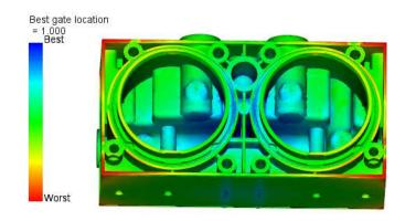
Figure 3.6: Gate analysis with the gate region locator method
