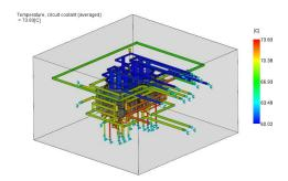
(b) Temperature of the coolant, averaged along the cooling channel path for the FEM analysis with automatic time
