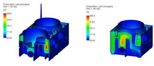
(b) Temperature, part (averaged): section 1, highest averaged temperature area
