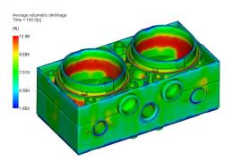
Figure A.4: Average volumetric shrinkage of the piece. Here the maximum shrinkage found is 12.38% while in the prior analysis it was 11.89%.
