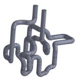
(b) Single conformal cooling channel
