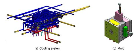
Figure 1.6: Solidworks file geometry view of the cooling channels and mold defined by the company for the piece under study.
