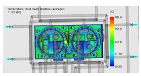
(a) Temperature, mold-cavity interface (averaged) result for Averaged within cycle with automatic time analysis
