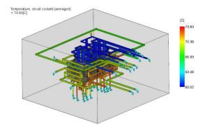
(b) Temperature of the coolant, averaged along the cooling channel path  $% \left( {{{\bf{n}}_{\rm{c}}}} \right)$
