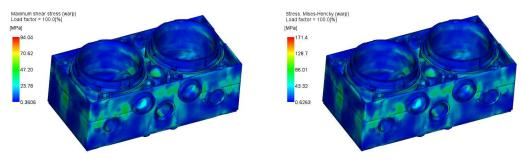
(a) Maximum shear stress, for brittle materials
