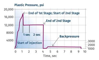
Figure 3.14: How an injection pressure plot should look like in an analysis and how it should also look in a real production run. (unit in psi) [30]
