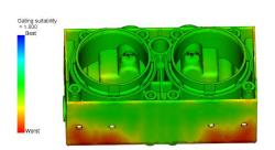
(a) New gate location analysis after the alteration of the piece's geometry. The best location, which should be represented in blue, can't be found.
