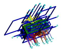
(a) Representation of the measuring procedure for the channels from the Solidworks file. Procedure to acquire the coordinates of the initial point for the channel.
