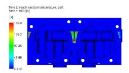
(a) Time to reach ejection temperature
