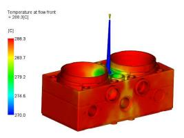
(a) Initial result at 260  $^{\circ}\mathrm{C}$  and original geometry for the sprue
