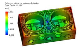
(c) Warpage due to differential shrinkage
