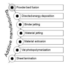
Figure 2.6: Additive manufacturing process categories according to ISO/ASTM 52900:2015. [18]
