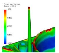
Figure A.3: Frozen layer fraction. Sprue detail at time 10.29 s of the cycle. The sprue is still only 50% frozen along its length, and the gate is still open for filling, but the injection nozzle at the machine-mold interface has already frozen.
