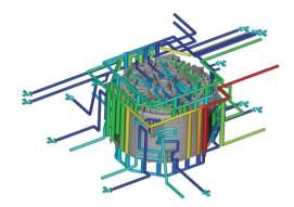
Figure 4.10: Correct representation of the average coolant temperature inside of a baffle. In the picture, multiple baffles can be seen, and the temperature is found to be uniform in the baffles as it is supposed to be. [36]
