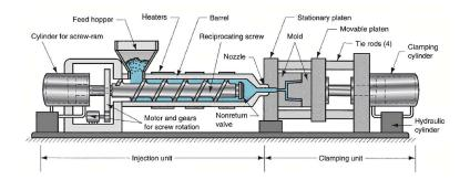
Figure 2.1: General scheme of the structure of an injection molding machine, single screw. [2]
