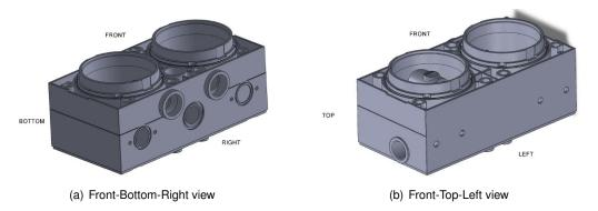
Figure 1.3: Perspective view of the piece from two different angles. Emphasis is given in these views to show the filter seats on what is called the front side of the piece.
