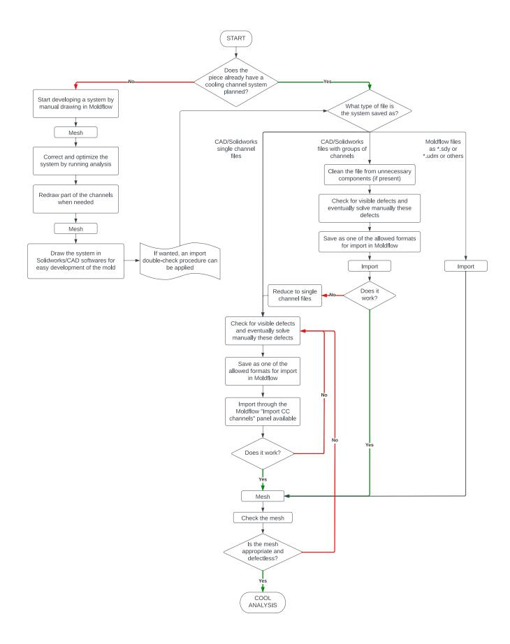
Figure 5.1: Flowchart scheme for the available import procedures for the cooling system.
