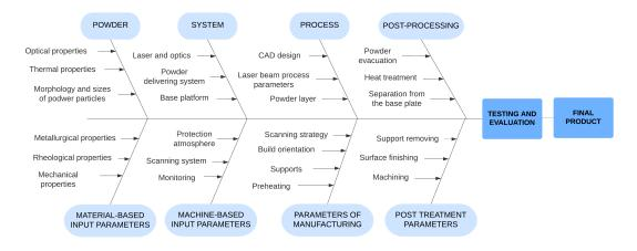
Figure 2.8: Main parameters influencing the quality of LPBF components, divided by categories. [18]
