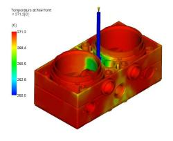
(c) Increase the diameter of the sprue, temperature at 260  $^{\circ}\mathrm{C}$
