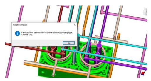
Figure 4.5: Change property for the imported channels before the mesh. This passage can be achieved by >select the complete geometry of one channel >right click on the selected area >change properties >channel or 3D channel.
