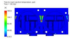
(b) Time to reach ejection temperature from the FEM analysis. The same orientation of the previous is used.
