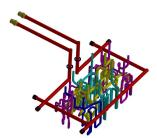
(a) Cooling system on the fixed side of the mold
