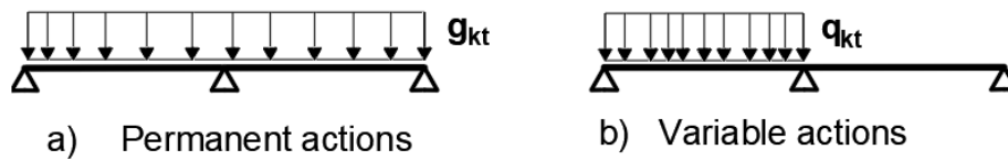
Figure 2.7. Disposition of actions for SLS deflection verifications of a slab
