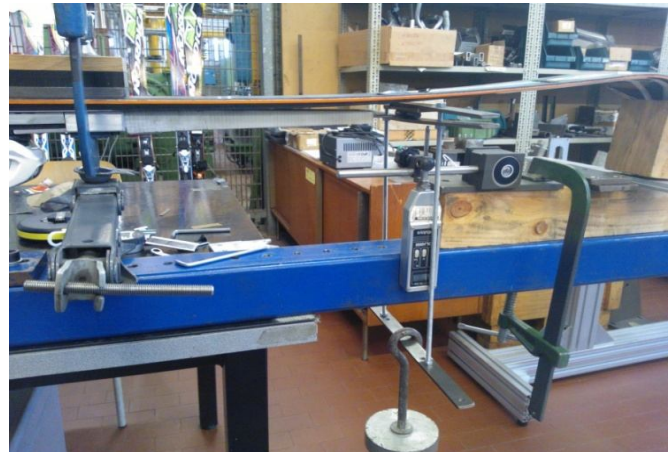
Fig. 23: Resin arm loaded on ski
