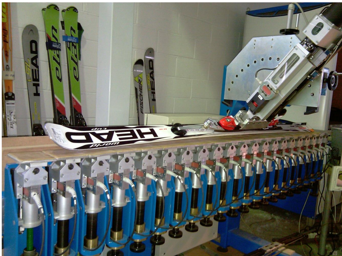
Fig. 40: Slytech bench, old configuration, 40 degrees inclined
