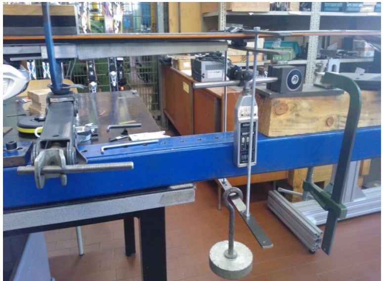
Fig. 26: Ski and resin arm loaded
