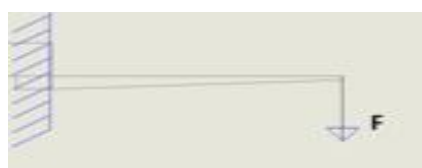
Fig. 78: Beam static model
