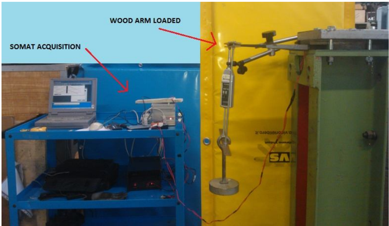
Fig. 34: Global view of wood arm loaded and data acquisition
