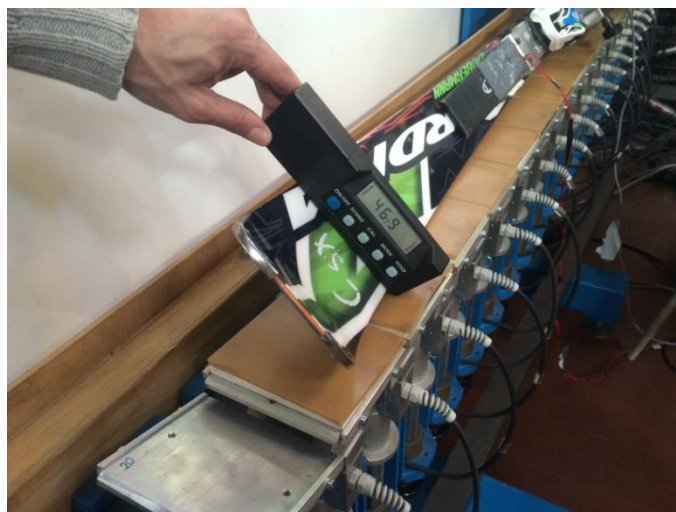
Fig. 59: Use of inclinometer for shovel torsion
