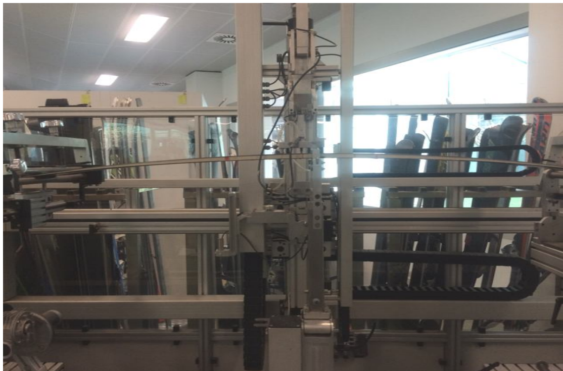
Fig. 63: Example of ski clamped and loaded on Nordica Flex Bench
