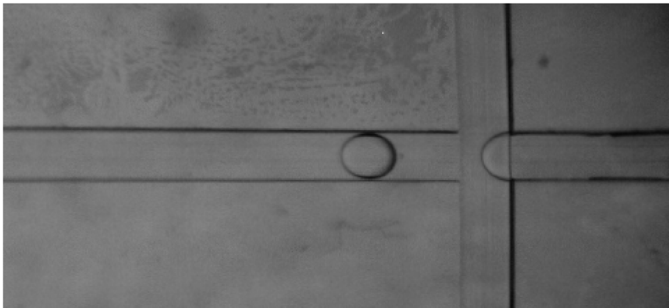
(a) Shape of the droplet soon after the formation in the T-junction.
