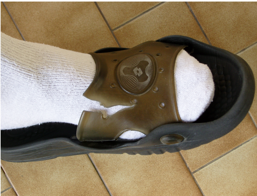
Ghost Figure. Multiaxial fatigue crack propagated inside a viscoelastic material component (the author's slipper).
