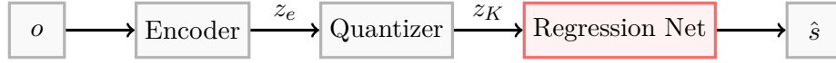
Figure 5.2: Pipeline for testing the performance of the semantic problem for different size of codebooks K .
