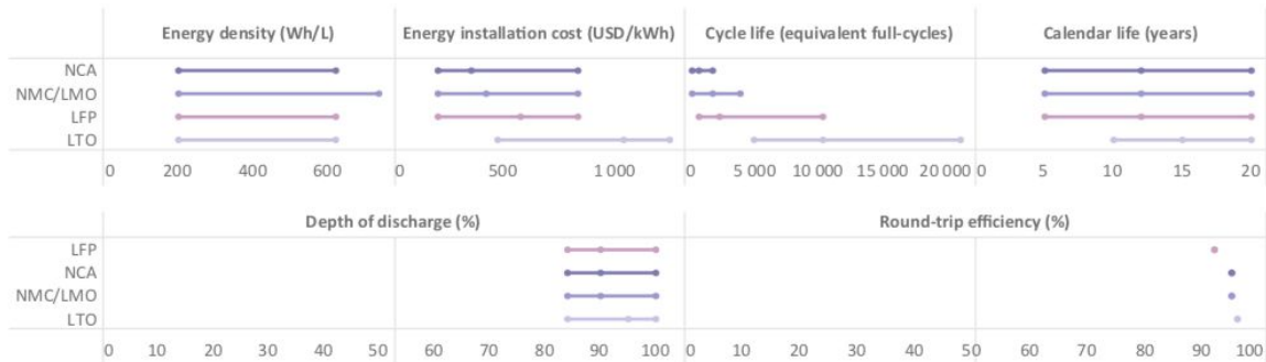
Figure 22 - Properties of selected chemistries of Li-ion ESS - Source [12]
