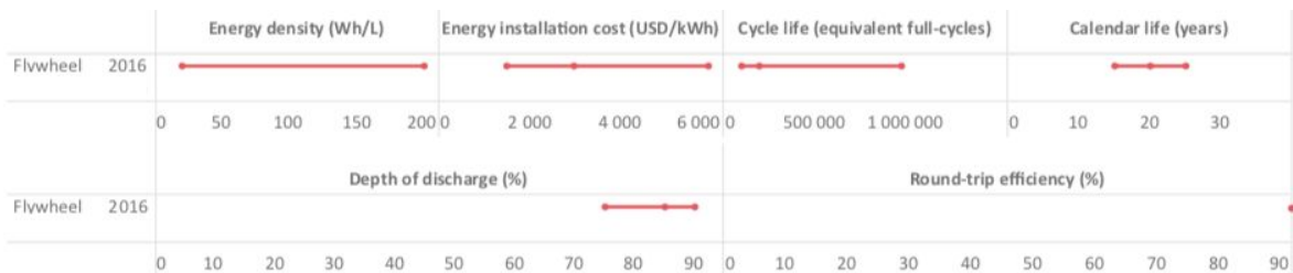
Figure 30 - Properties of flywheel energy storage systems - Source [12]
