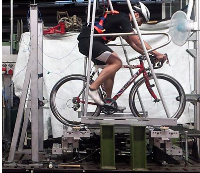
Figure 3.7: Test bench with front and rear rollers shaking made by Mattia Scapinello
