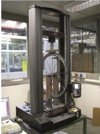
Figure 3.1: Campagnolo® wheel test bench[9]
