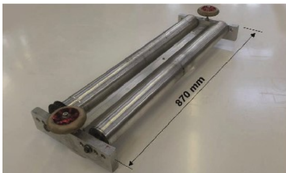
Figure 2.1: Wider roller shaker
