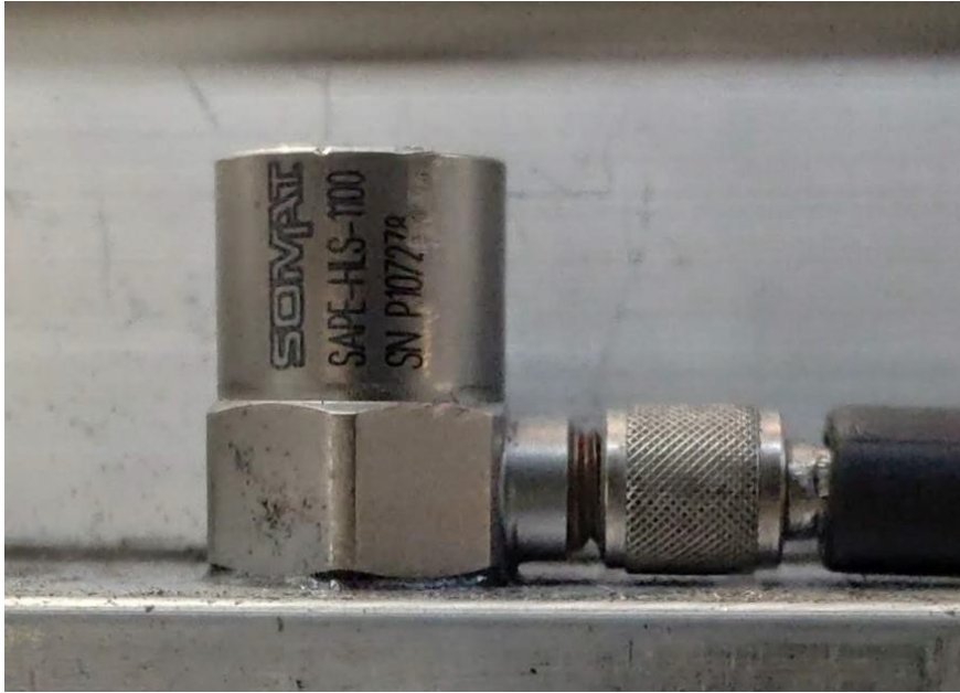
Fig 2.13 Detail of Uni-axial piezoelectric accelerometers
