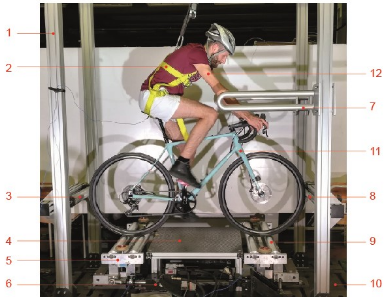
Figure 3.8: Test bench with front and rear rollers shaking improved By Enrico Girlanda
