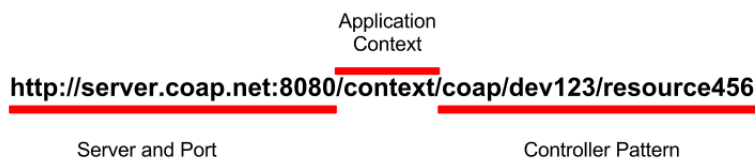
Figure 2.1: An example of HTTP URL that can be handled by a controller
