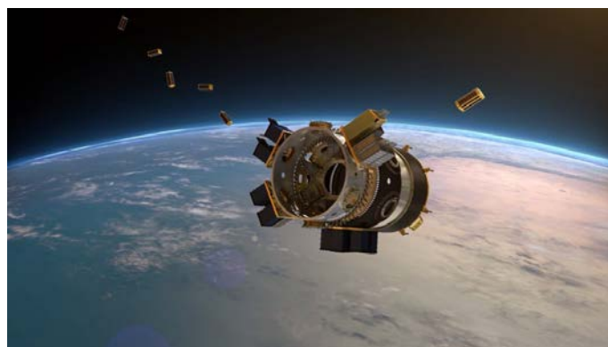
Figure 1.2: A complete deployment system by SpaceX with many deployers attached, rendered during the release of the satellites into orbit. Digital rendered image. Released by SpaceX. 2018.
