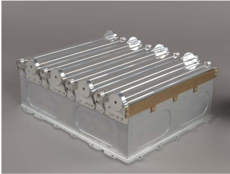
Figure 4.1: The classical structure of a louvers designed for a large spacecraft, composed of several independently moved blades. Louvers, Temperature Control System, Mariner 2. Digital image. Smithsonian - National Air and Space Museum.
