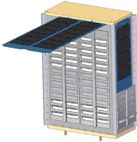
Figure 4.2: The passive louver for CubeSats developed and patented by NASA. Digital image. NASA CubeSat Form Factor Thermal Control Louvers. NASA Technology Transfer Program.
