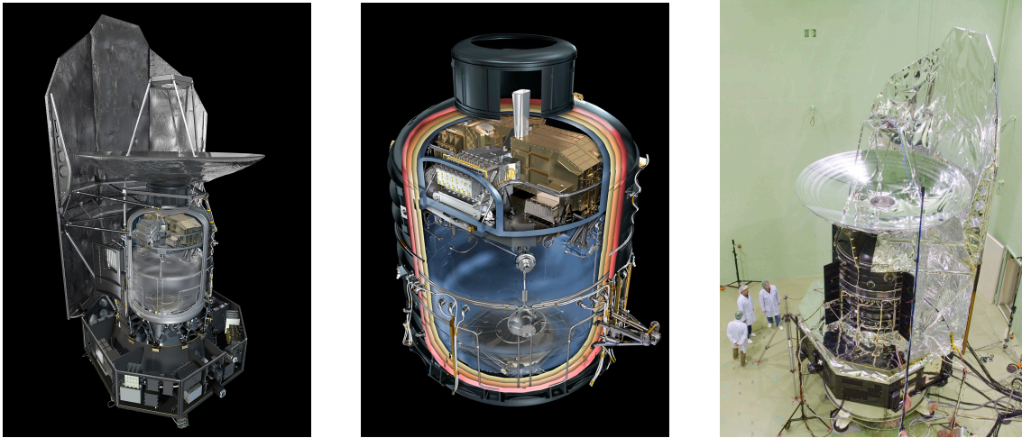
Figure 2.2: Left: The Herschel spacecraft features the ‘payload module’ (PLM) with the cryostat housing the instrument focal plane units (FPUs), the telescope, the ‘service module’ (SVM) with ‘warm’ electronics, and the sunshield/sunshade. Middle: Close-up of the PLM displaying the optical bench with the instrument FPUs on top of the main helium tank. The focal plane cover and the three vapour-cooled shields inside the cryostat vacuum vessel (CVV) are also shown. Right: Herschel being prepared for acoustic testing in the Large European Acoustic Facility (LEAF) in the ESTEC Test Centre in June 2008, providing a good view of the telescope (ESA).
