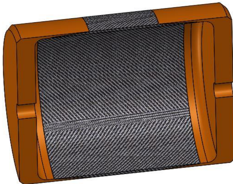
Figure 47. Scarf Joint Test Design
