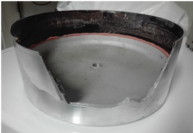
Figure 50. Scarf Joint Test Result
