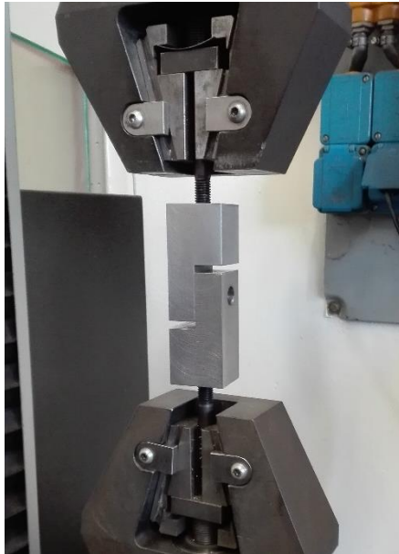
Figure 59. Screw Test Configuraiton
