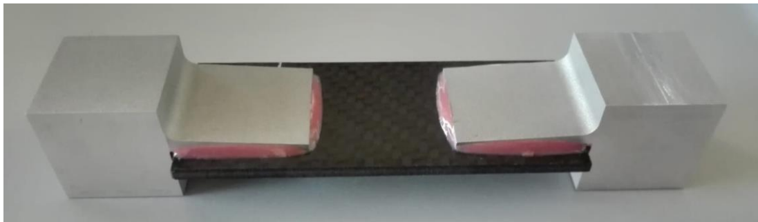
Figure 41. Strap Joint Assembly Result
