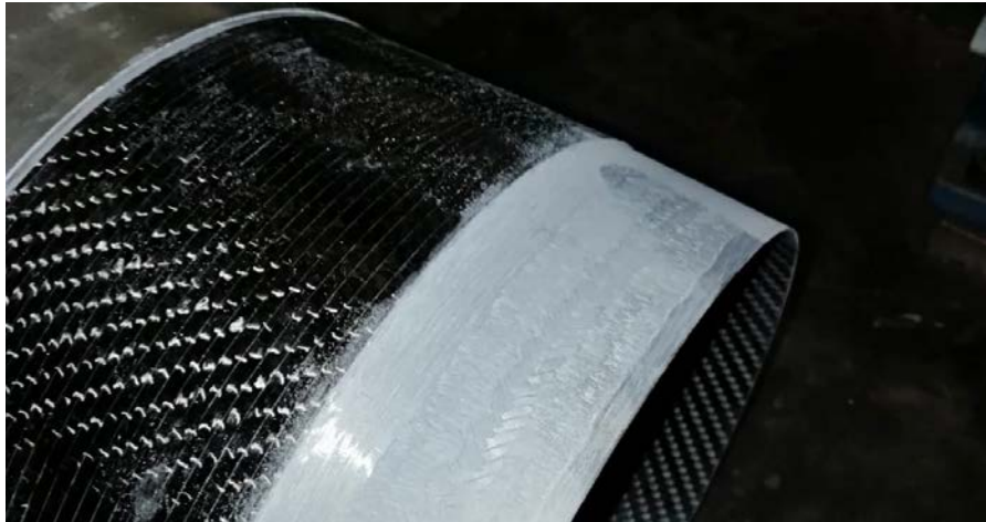
Figure 48. Scarf Joint Gluing Area
