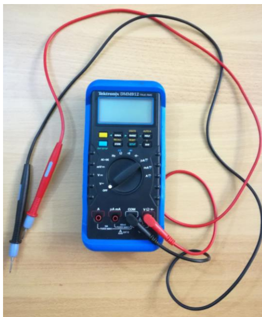
Fig. 37 - Digital multimeter that the students can use to take current and voltage measurements.
