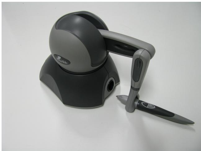
Fig. 2.2: Phantom Omni Device
