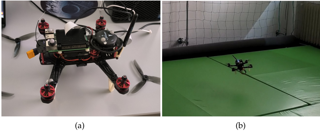
Figure 7.1: HolyBro QAV250 quad-copter: on a table without the propellers (a), during flight in the flying arena in the SPARCS lab(b).
