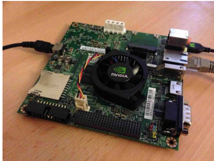
Figure 5.7: The NVIDIA Jetson TK1 is the rover core, exploiting a Tegra K1 SOC.
