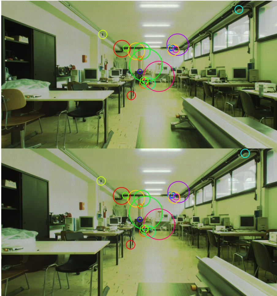
Figure 4.5: An example of left feature tracking between two instants using SURF detector and descriptor and Brute-force matcher. The circle radius around each keypoint indicates the size of the detected blob.
