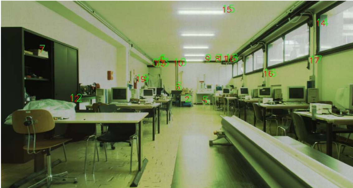
Figure 4.11: Example of 2D-3D correspondences after the outlier rejection steps. The red number indicates the 3D reprojected points on the left image plane, \hat{\mathbf{x}}_{k-1}^i , while the green ones are the corresponding 2D points, \mathbf{x}_k^i . The outlier rejection allow to remove almost all of the bad correspondences and thus to reduce the computational time of the motion estimation step.
