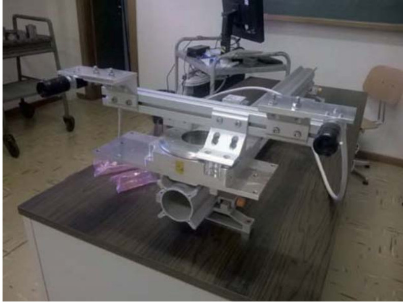
Figure 5.1: The experimental set-up used to record the datasets [34]. It comprises the stereo camera mounted on the rotary stage, which can translate along the linear slide.
