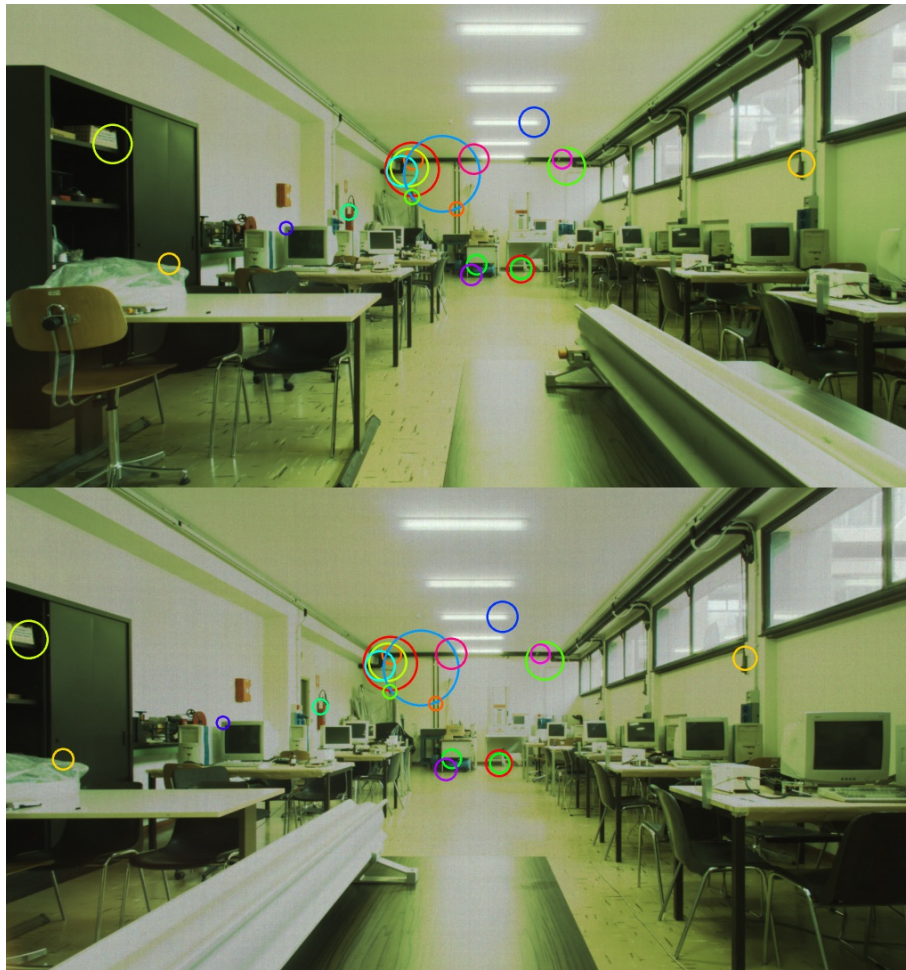
Figure 4.4: An example of left-right feature matching using SURF detector and descriptor and Brute-force matcher. The circle radius around each keypoint indicates the size of the detected blob.
