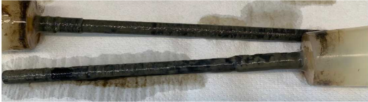
Figure 36 Presence of biofilm on the graphite electrode from reactor R1-1.0 V in experiment I, own representation.
