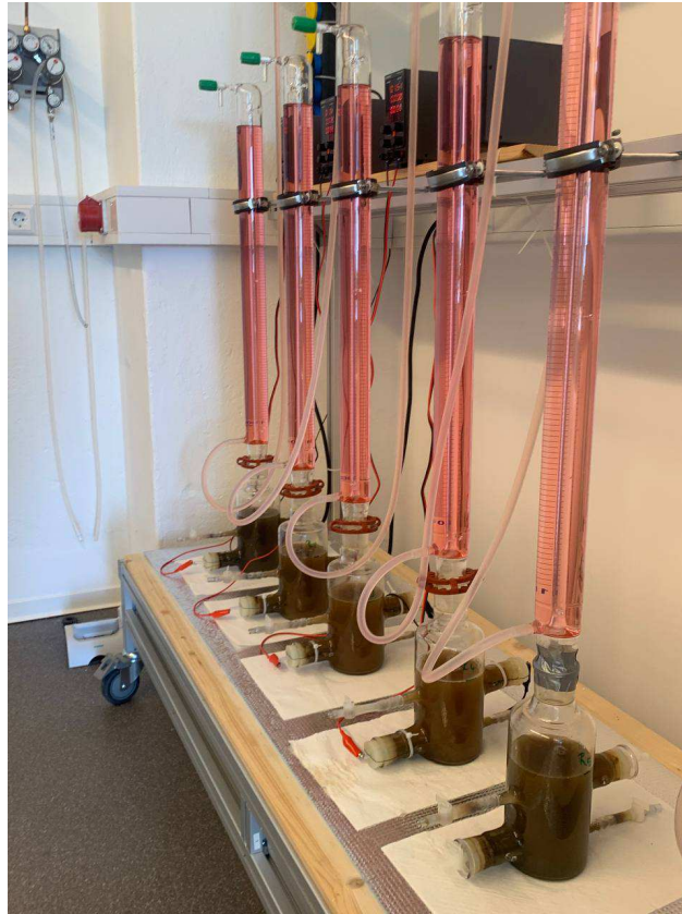
Figure 11 Eudiometer for determination of gas from substrate, own representation.
