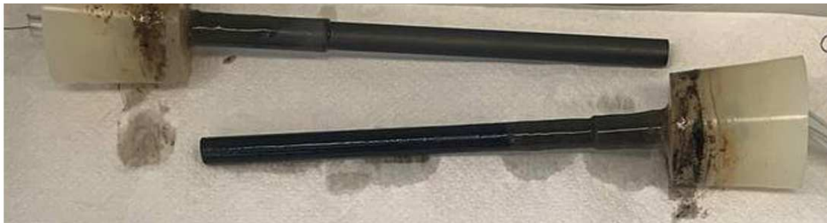
Figure 37 Presence of biofilm on the graphite electrode from reactor R2-1.0 V in experiment I, own representation.
