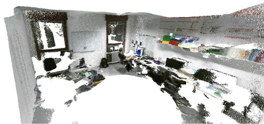
Figure 15: Reconstruction of the LTTM laboratory room made with the MICROSOFT KINECT FOR XBOX ONE range camera. The two pictures show the final point cloud from different points of view.
