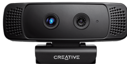
Figure 7: The CREATIVE SENZ3D range camera.
