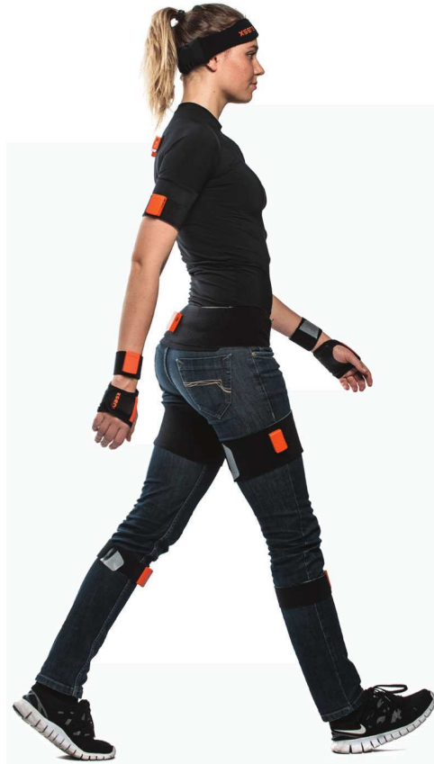
Figure 10: IMUs for biomechanical applications have been incorporated into MoCap suits (i.e., the XSENS MVM suit) [19].
