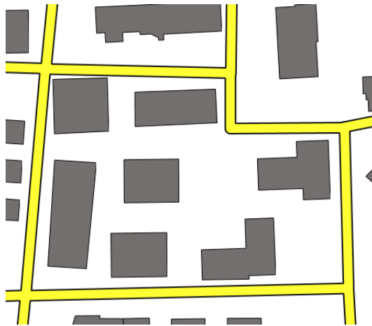
Figure 3.4: Biggest buildings are displaced over the available area while the smallest have been removed.
