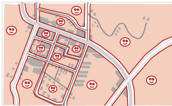
Figure 2.5: Using the road network to partition the map space in terms of responsibilities and activities between agents.
