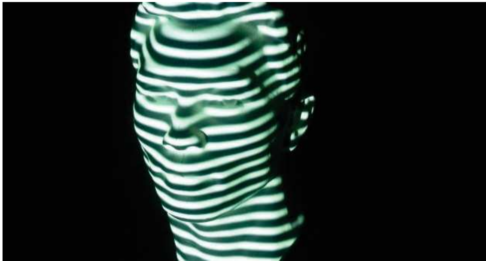
Figure 1.3: Use of structured light for 3D surface imaging
