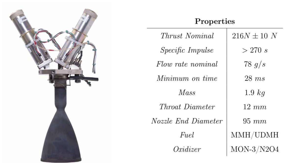
Figure 5.9: 200 N bi-propellant thrusters, courtesy of [16].
