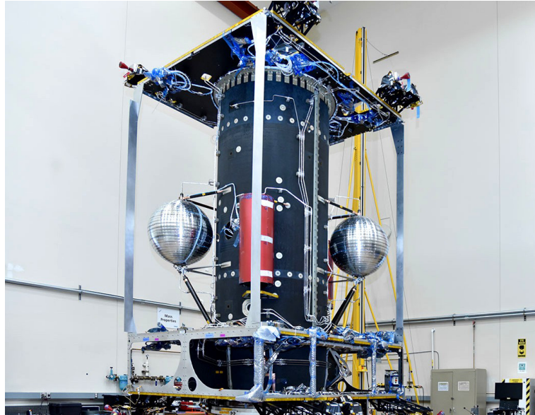
Figure 5.3: The basic structure of OSAM-1 being assembled (courtesy of [28]).
