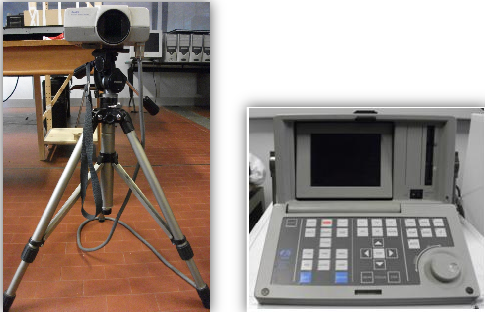
Fig. 3: Infrared camera: the camera detects the radiation that are transmitted and processed in the instrument display.
