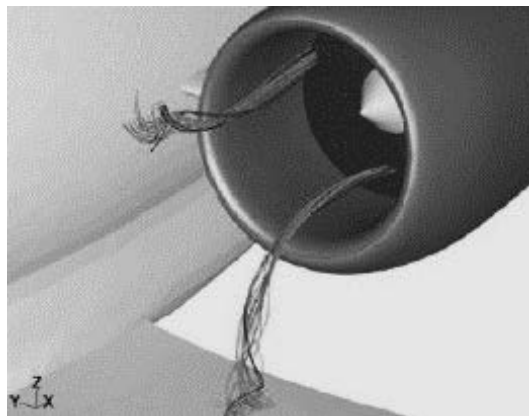
Figure 2.5: Tightly-wound vortex attached to airplane surface [7]
