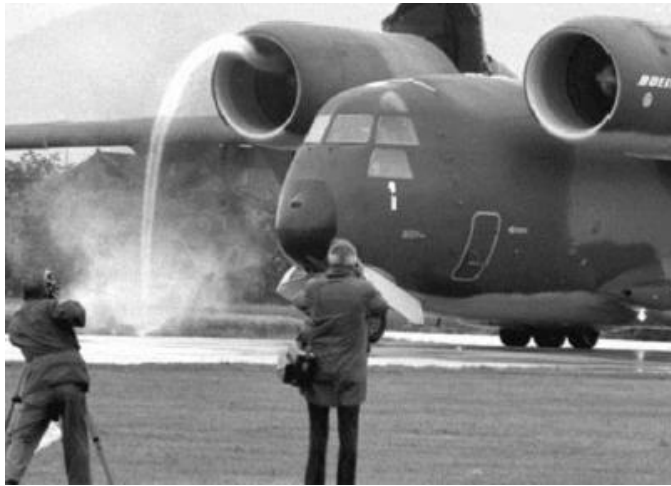
Figure 2.4: Tightly-wound vortex attached to the ground [7]
