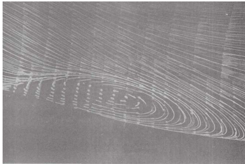
Figure 2.9: Close up of the surface oil flow patterns developed in the separation region [10]
