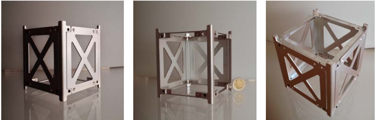
(a) Partially assembled CUBE structure. (b) Comparison between a 1U CubeSat structure and a 2 Euro coin. (c) Fully assembled empty CUBE structure.
