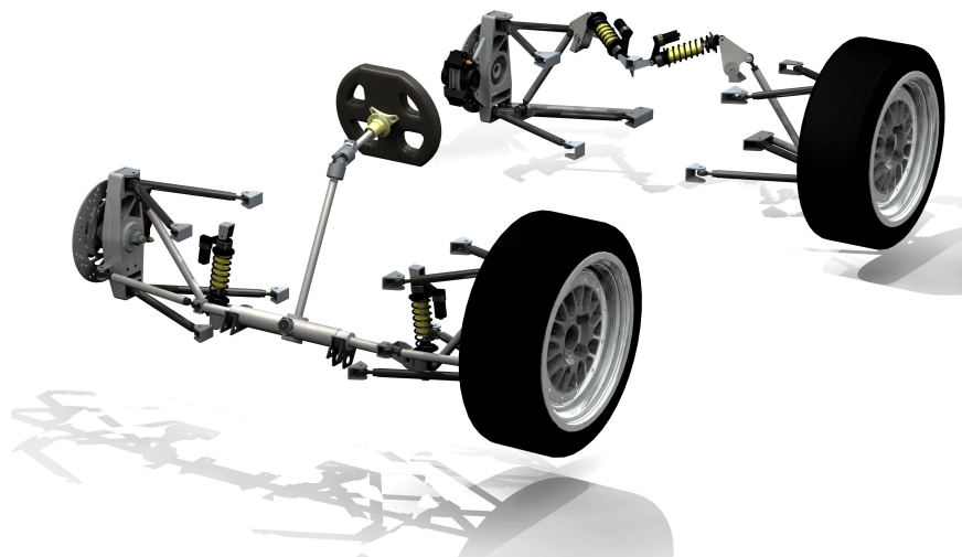
Fig. 2.7: 3D multibody simulator model of a car suspension and steering system
