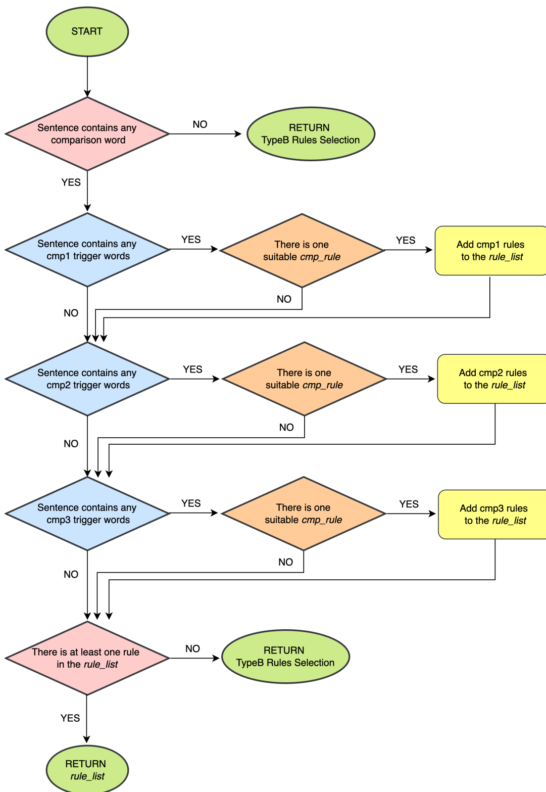
Figure 5.4: TypeA rules selection flow. We start by checking if the sentence contains any comparison word and then we check the rules applicability based on some trigger words and another function that returns the second part of the rule. We check applicability for each group of rules separately and in the end we check the rule_list content. If it is empty, we check for TypeB rules, otherwise we return the retrieved rules.
