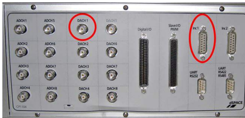
Figure 3.3 dSPACE DS1104 controller board: connectors panel
