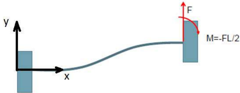
Figure 2.8 General single deformed compliant sheet/beam
