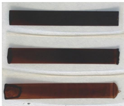
Figure 3.4. The comparison between the slot-die deposition of three different formulation: original ink (left); Ink diluted at 50% in volume of ink (middle); ink diluted at 75% in volume of ethanol (right). It can be observed an increase of light-brown coloration with the increase of solvent content and reduction of solid particles.
