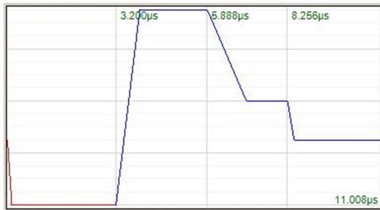
Figure 3.2. Characteristic voltage waveform utilized for the inkjet printing deposition. This particular shape enabled to achieve an optimal jetting behavior.
