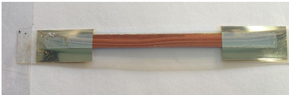
Figure 4.8. The configuration of the sample utilized for evaluating the performance of the copper electrodes. The non-covered part is 5 cm long, while the silver edges are around 1.5-2 cm large.
