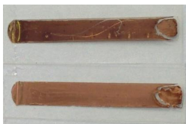
Figure 4.4. Samples exposed to oxygen: comparison between a one-step approach (top) and a two-steps process (down).
