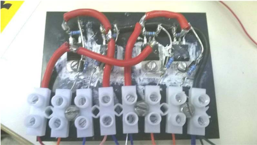
Figure 10.1.3 – The H bridge circuitry
