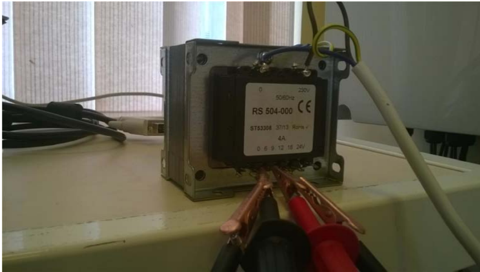
Figure 10.2.3 – Single phase transformer, the primary winding connected to the grid (upper wire) and the secondary winding connected to the AC/DC converter and the dSPACE platform as an analogic signal source.
