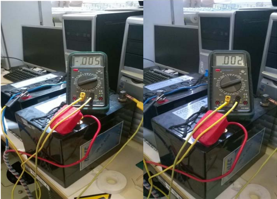
Figure 10.2.6 / 10.2.7 – The picture on the left shows a negative current, so a current which is absorbed by the battery, according to the conventions used. The picture on the right shows a positive current, which means the discharging of the battery.
