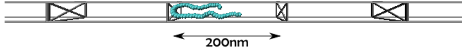
Figure 4.2: Backfold of a linear chain of N = 50 beads in a channel of width \Delta = 32.7 nm.
