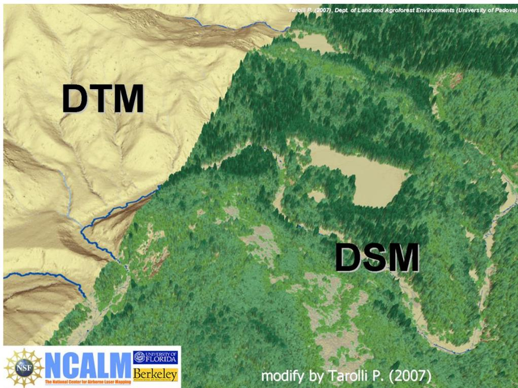
Figura 1.2.1: Differenze tra DTM e DSM (modified by Tarolli, 2008).
