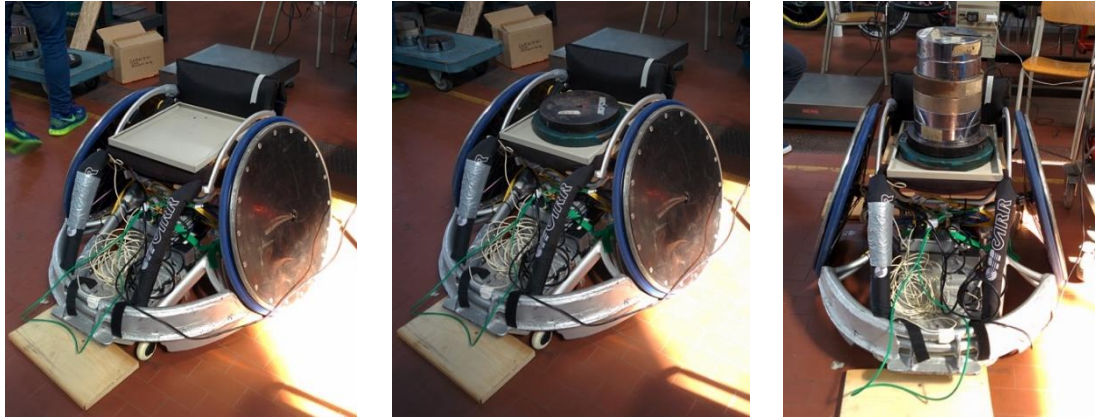
Figure 4.8: Setup of vertical calibration
