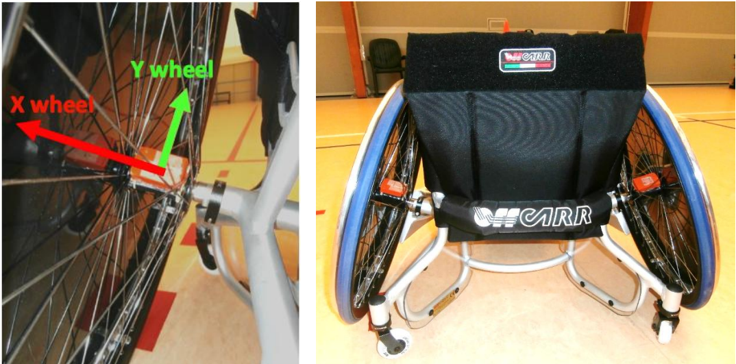
Figure 6.4: Sensors in the wheels. Left: wheel system of reference; right: sensors fixation.
