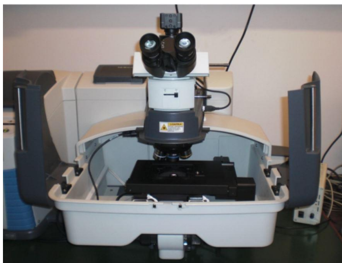
Figure 2.2. The Micro-Raman spectrometer (Thermo Scientific DXR MicroRaman) located at DISC, University of Padua.
