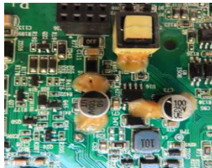
Figure 4.46: Power Supply Block
