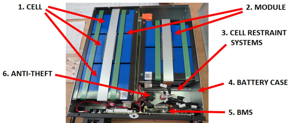
Figure 4.27: Internal of Battery Pack n.2
