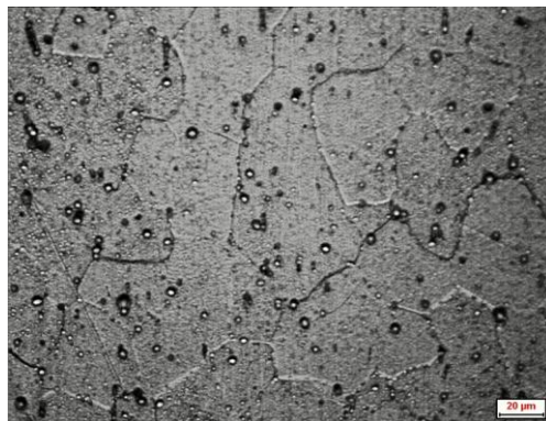
Figura 25 - Micrografia AA6016 - T_f=510^{\circ}\text{C}
