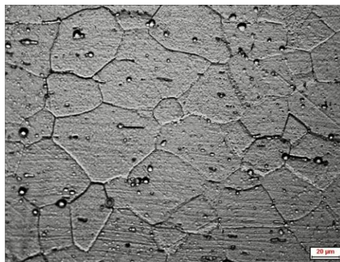
Figura 26 - Micrografia AA6016 - T_f=550^{\circ}\text{C}
