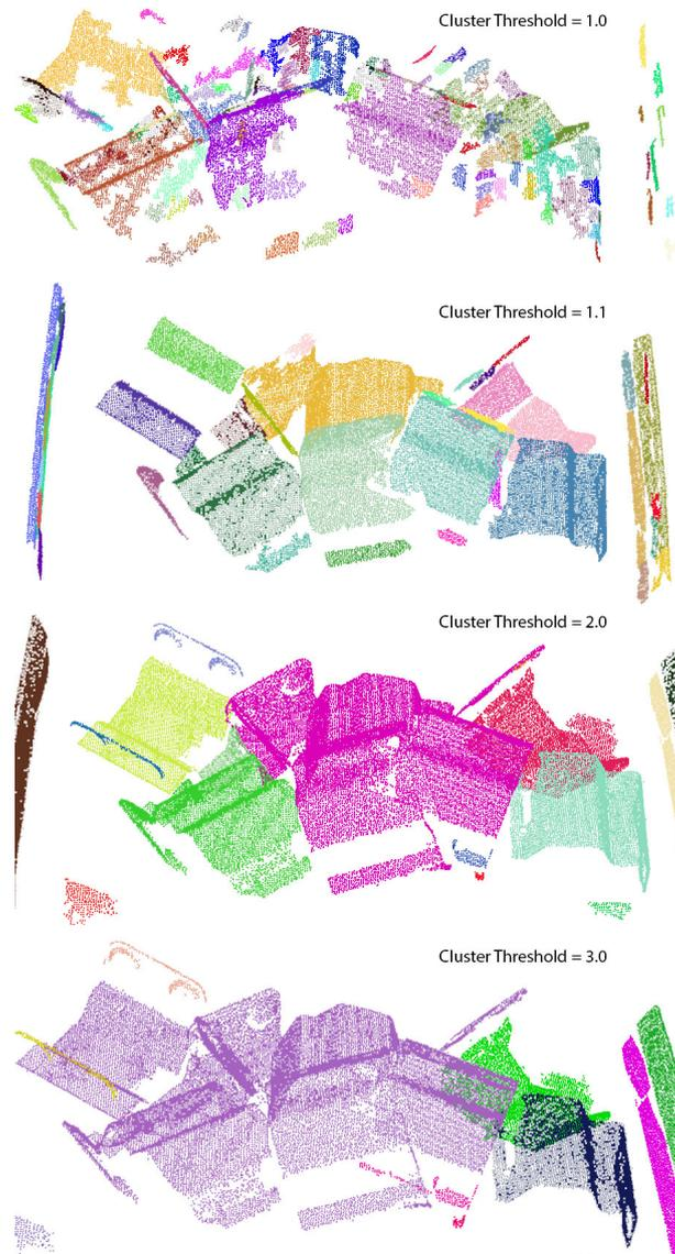
Figure 3.18: Clustering of the same cloud (resolution=1.0mm) with different tolerances:
