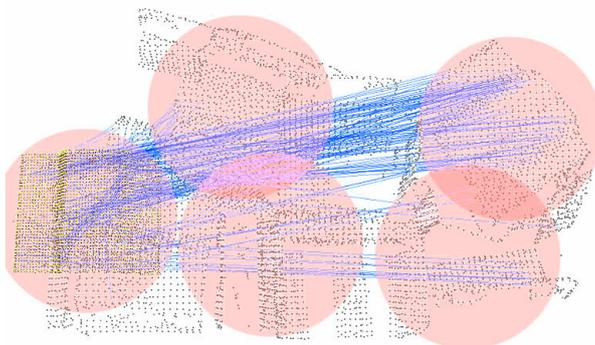
Figure 3.17: Correspondences found using spheres of world cloud. The key idea is that a good set of correspondences can not be larger than the object size.
