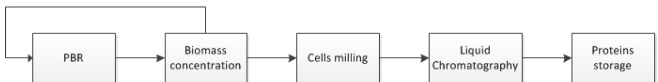
Figure. 4.1. A Block Flow Diagram of the process to produce microalgae aimed to protein recovery.
