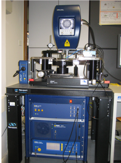
Figura 3.26: Profilometro Polytec MSA-500
