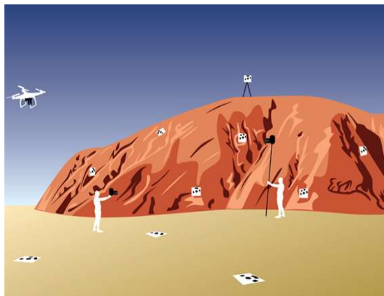
Figure 2.13. Scheme of SfM survey and the position of targets on the ground. Source: www.unvaco.org
