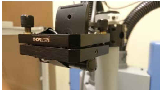
Figure 3.19: Mechanical tool used to keep the camera fixed
