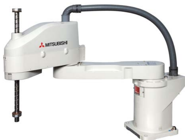
Figure 2.1: Example of SCARA robot
