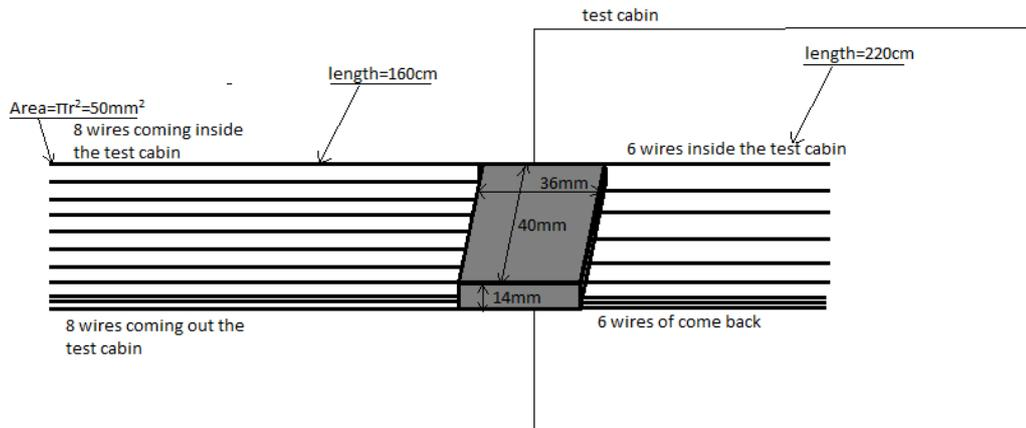
Figure 4.16 - Wires of connection to the test cabin from the bank-circuit
