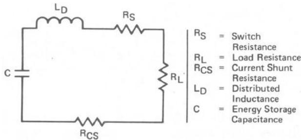
Figure 6.2 - Equivalent RLC circuit
