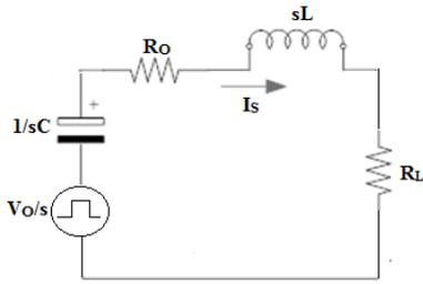
Figure 6.4 - Equivalent RLC circuit with Laplace-Transformation for each electric component
