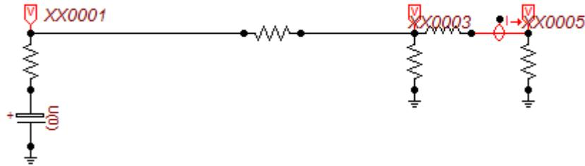
Figure 5.10 – ATP simplify scheme for the D-bank's circuit
