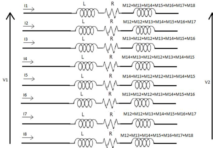
Figure 6.17 - Simplify equivalent electric scheme for the eight wires taken from the equation (6.17-6.18)
