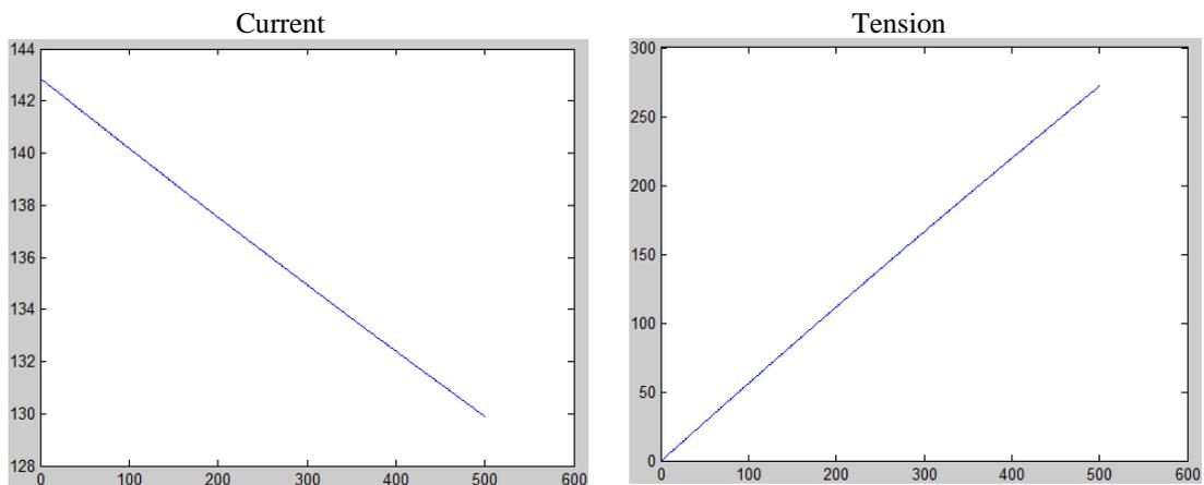
Figure 5.16 - Matlab plot of current and tension in the capacitor of the C-bank during the charging
