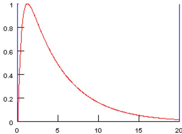
Figure 4.6 - Shape of switching current in the A-B-D Bank
