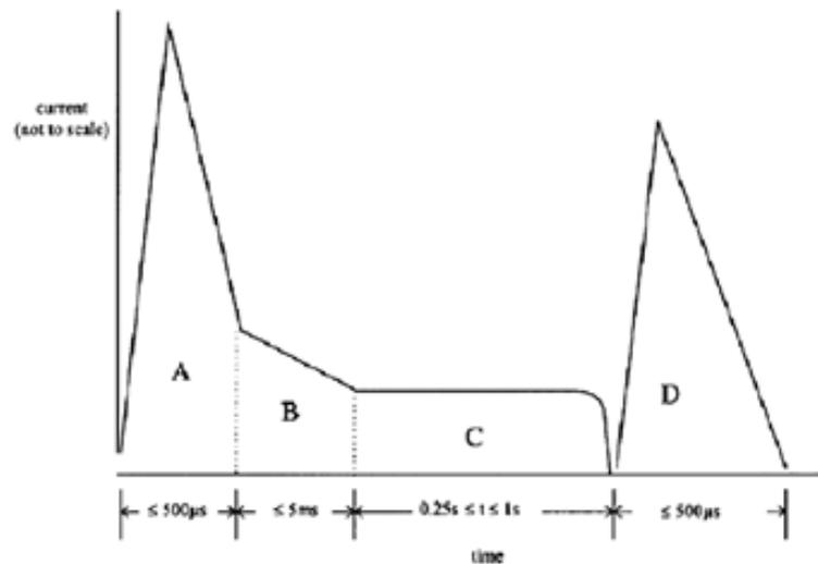
Figure 4.3 - Complete waveform of the 4 bank of capacitor
