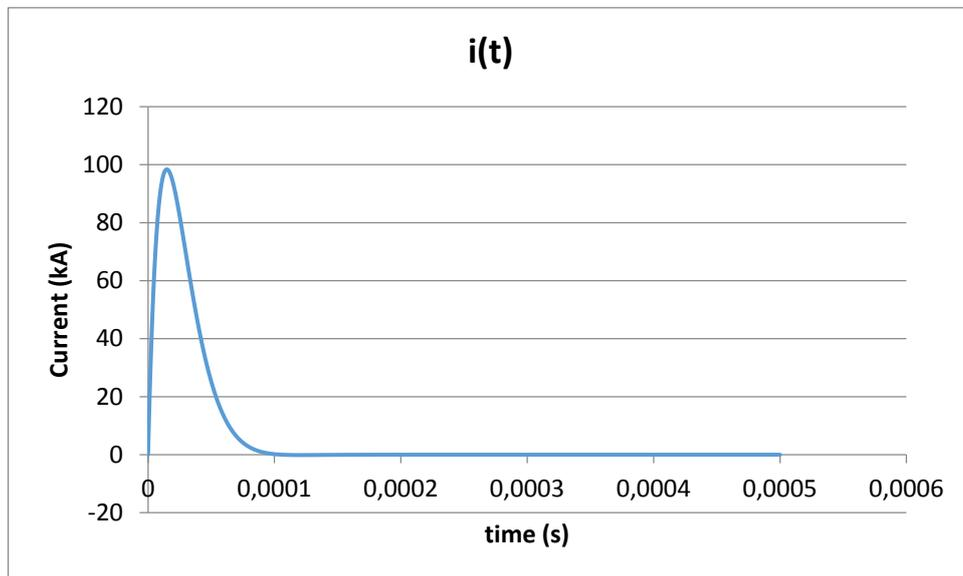
Figure 6.5 – Excel plot of  $i_s(t)$  for a negative “ $\Delta$ ” value in the equation (6.5)
