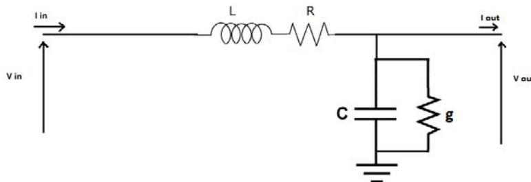
Figure 6.7 - Wires of connection to the test cabin representation with distributes electric component
