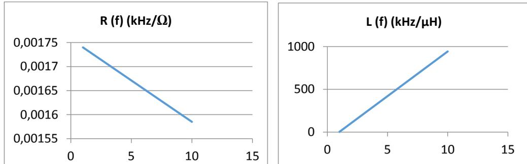
Figure 6.30 – Graphic representation of resistance's and inductance's values in function of the current's frequency applied to the power line (resistance's components before the cables)
