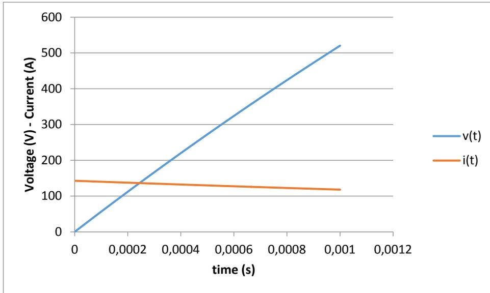
Figure 5.17 - Excel plot of current and tension in the capacitors of the C-bank during the charging
