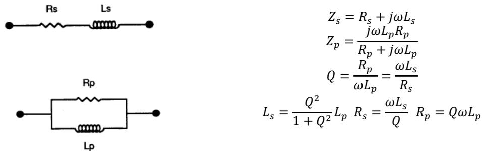
Figure 6.31 - Resistance's and inductance's model used by the LCR400
