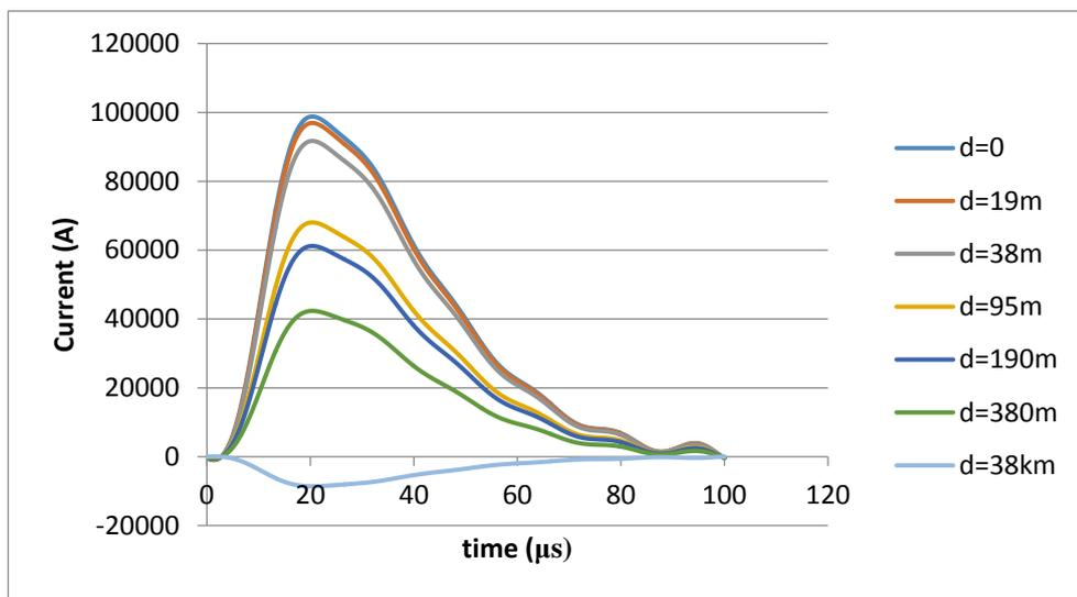
Figure 7.14 -  $i(x,t)$  Current's shapes for different hypothetical distance in a cable of the figure 7.13 corrected from the initial errors made by FFT approximation of the original current  $i(t)$  sampled
