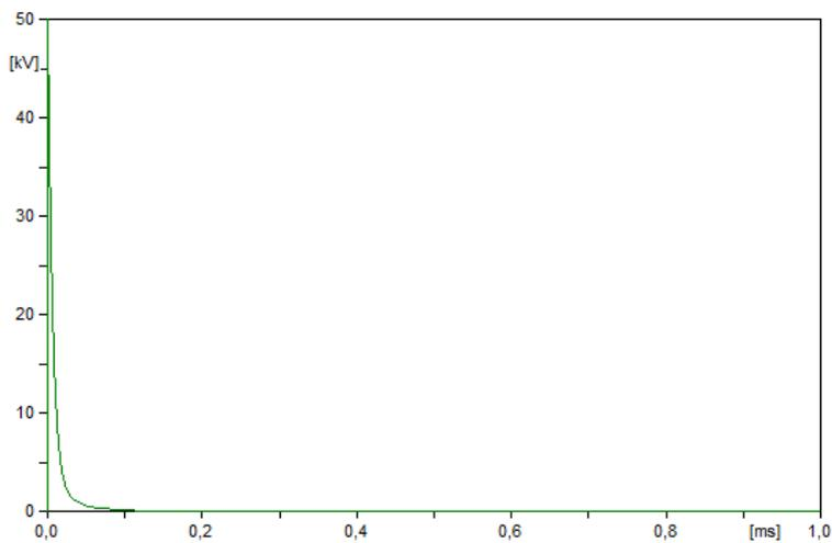
Figure 5.6 - Plot of the Voltage XX0004 that come from the ATP simulation
