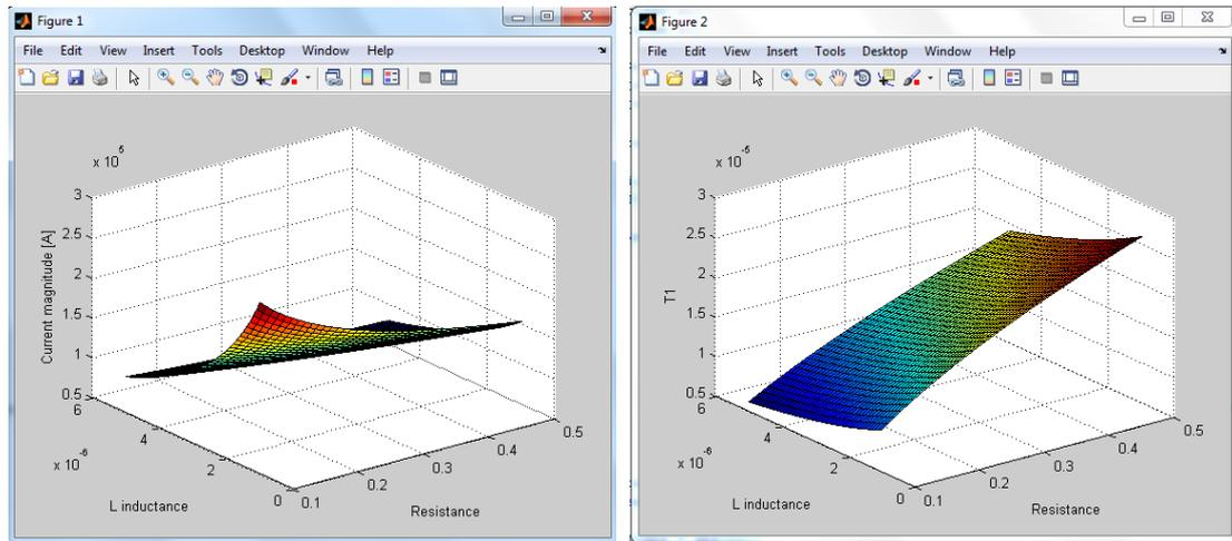
Figure 6.8 – 3D Matlab plot of  $is(t) = f(L, Rl)$  and  $T_{max} = f(L, Rl)$  functions
