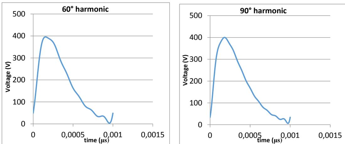
Figure 7.9 - Tension's shape by using the FFT series representation (stopping at the 60<sup>th</sup> harmonic/90<sup>th</sup> harmonic, in excel, with a jump of 10 harmonics each step)
