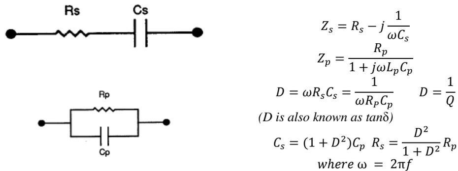
Figure 6.32 - Resistance's and capacitor's model used by the LCR400.
