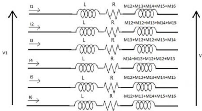
Figure 6.18 - Simplify scheme of the six wires that came from the equation (6.22)
