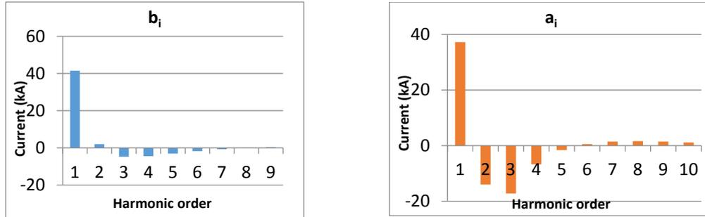
Figure 7.5 – Harmonics current's values' diagram for the “ $a_i$ ” and for the “ $b_i$ ” (FFT terms)
