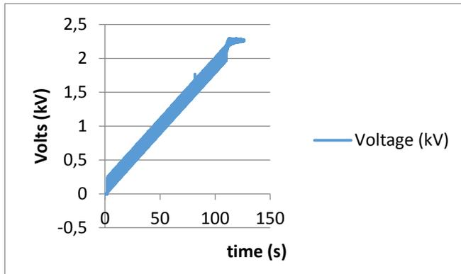
Figure 5.20 – Shape of tension (in 6 of the 13 capacitors) during the charging of the C-Bank with the capacitor filter (oscilloscope sampling)
