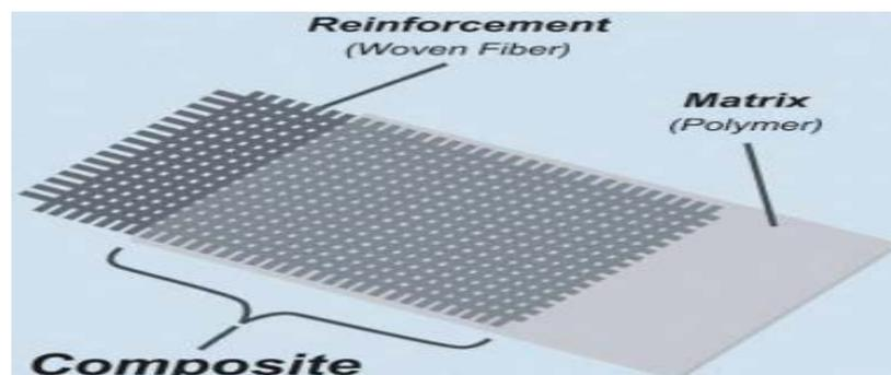
Figure 1.3 - Composite material
