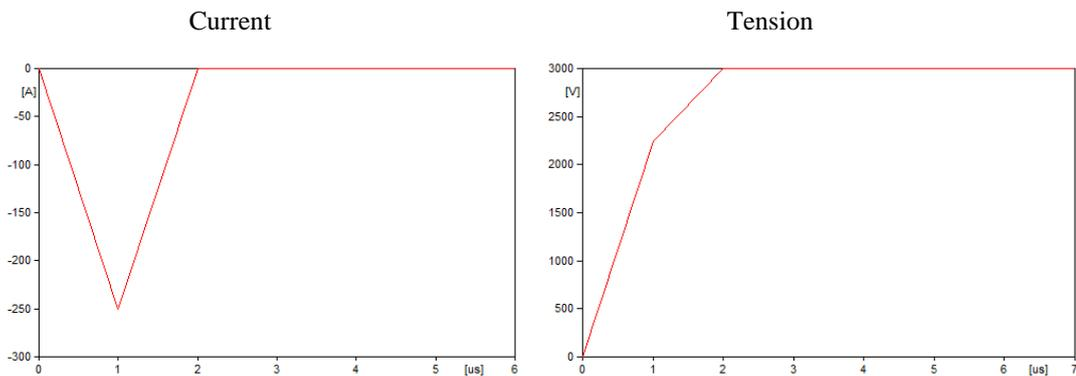
Figure 5.15 – ATP plot of current and tension in the capacitor of the C-bank during the charging
