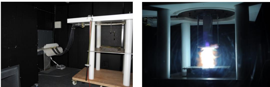
Figure 4.18 - Finally electric arc used for testing material inside test cabin. This picture is made with a particular photo machine that has inside, a kind of stroboscope, necessary for capture the electric arc's moment
