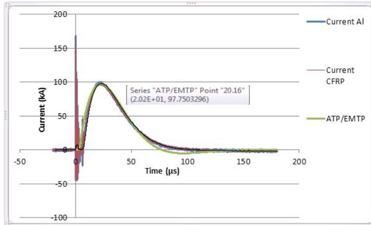
Figure 5.12 – Excel graphic comparison between ATP (with  $L=4,4\mu F$ ) and the sampling values form the testing of the aluminum's material
