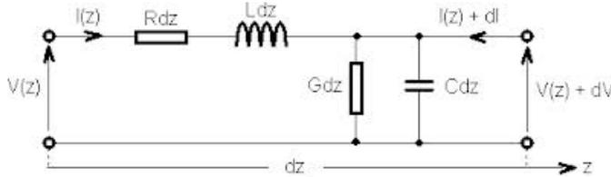
Figure 6.33 - Electrical elements of a power line (represented by concentrate constants)
