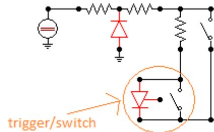
Figure 4.7 - Trigger switch in the C-Bank
