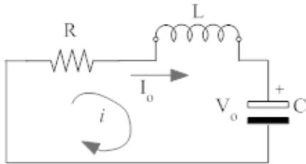
Figure 6.3 - Simplify RLC equivalent circuit
