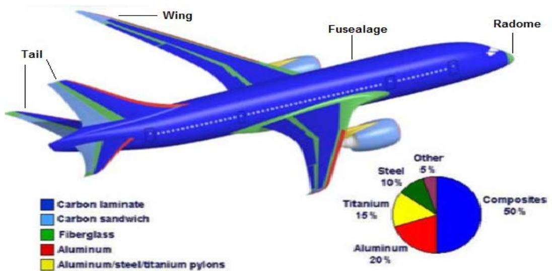
Figure 1.2 – Metals and composite materials used in the Boeing 787 Dreamliner
