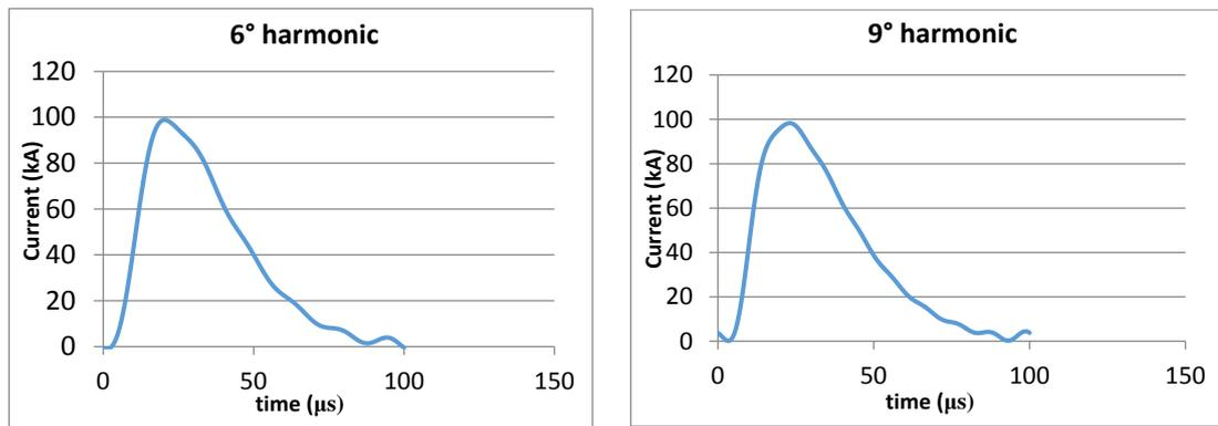
Figure 7.6 – Current's shape by using the FFT series representation (stopping at the 6° harmonic/9° harmonic, in excel)
