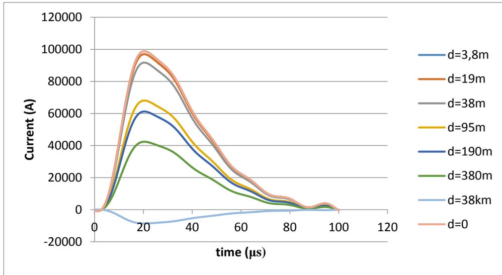
Figure 7.13 -  $i(x,t)$  Current's shapes by plotting in excel the equation 7.8 for different hypothetical distance ( $d, 5d, 10d, 25d, 50d, 100d, 1000d$ ) in a cable (" $d=3,8 \text{ m}$ ")
