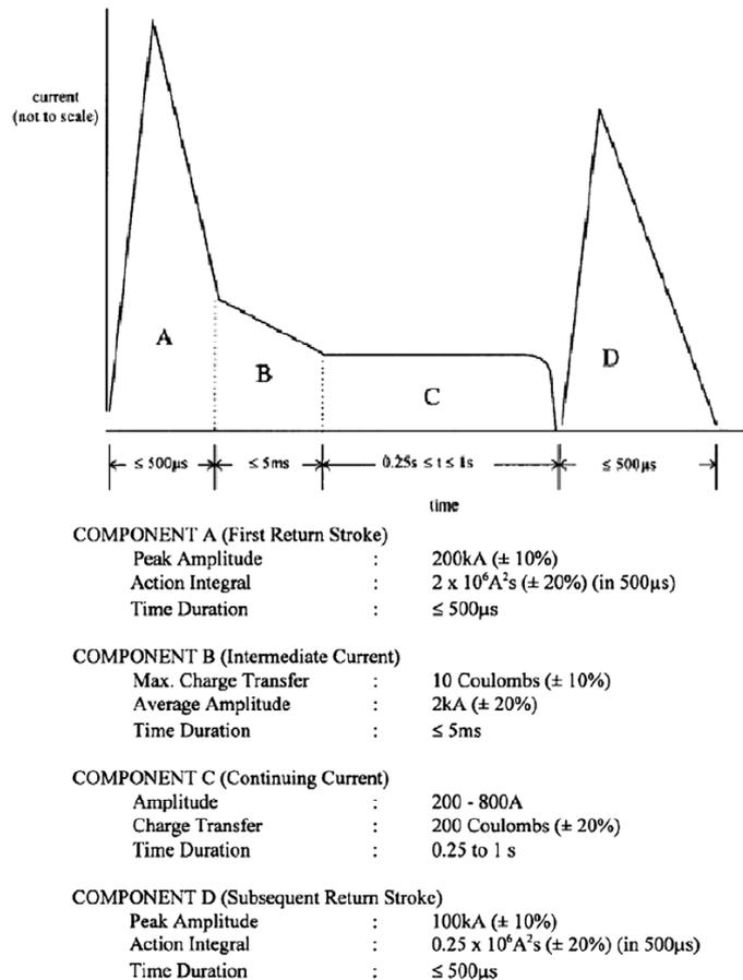
Figure 5.1 - Complete waveform of A,B,C,D-bank and their main parameters
