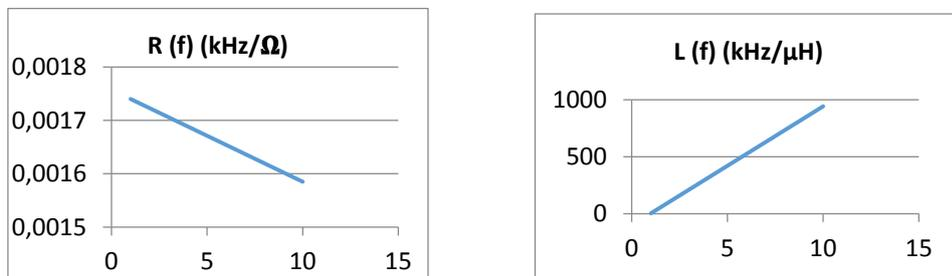
Figure 6.26 – Graphic representation of resistance's and inductance's values in function of the current's frequency applied to the power line (outside the test cabin)
