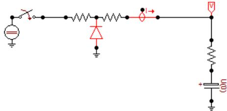
Figure 5.14 - ATP capacitor's charging scheme
