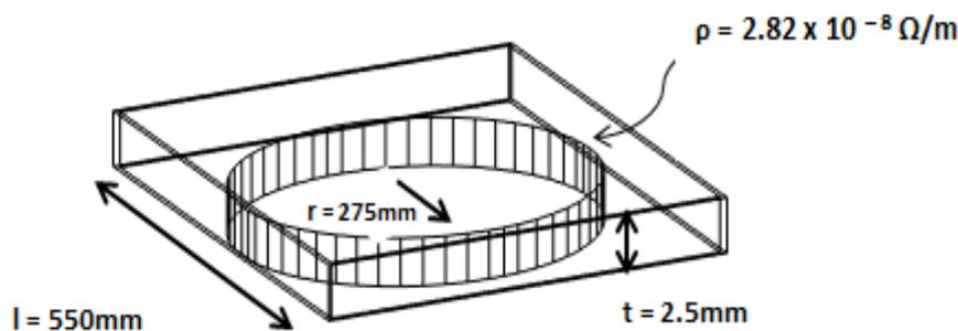
Figure 6.10 - Geometry of the aluminum panel
