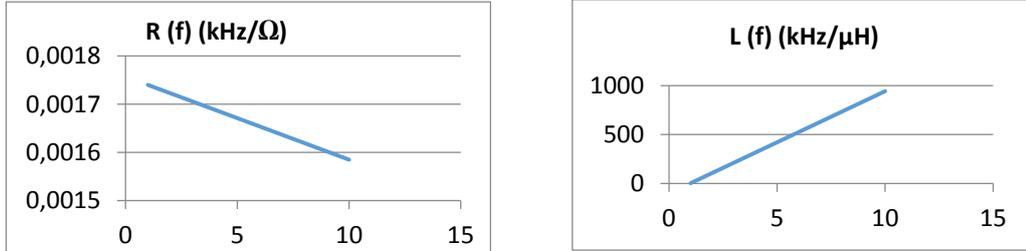
Figure 6.25 - Graphic representation of resistance's and inductance's values in function of the current's frequency applied to the power line (inside the test cabin)
