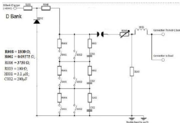
Figure 4.2 - D-bank circuit scheme
