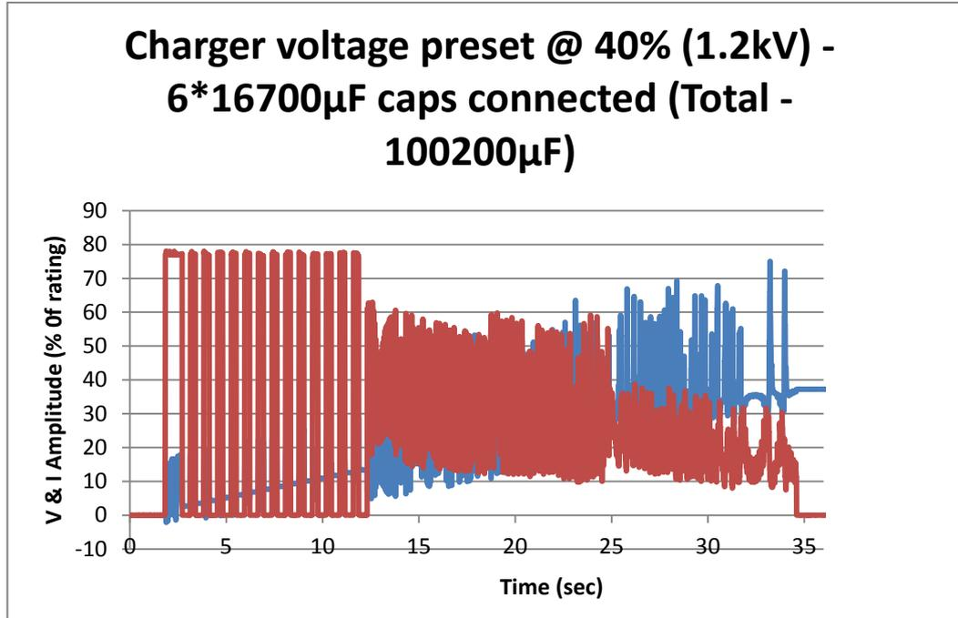
Figure 5.18 – Shape of current and tension (in 6 of the 13 capacitors) during the charging of the C-Bank (oscilloscope sampling)
