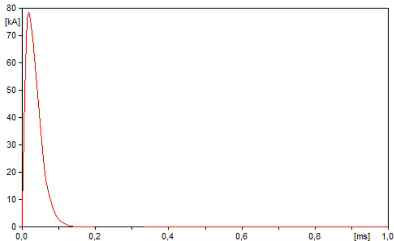
Figure 5.11 – Current's plot by ATP simulation for the D-bank's circuit.
