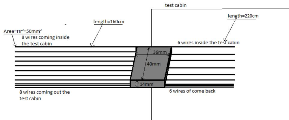
Figure 6.11 - Geometry of the eight/six wires of connection to the test cabin
