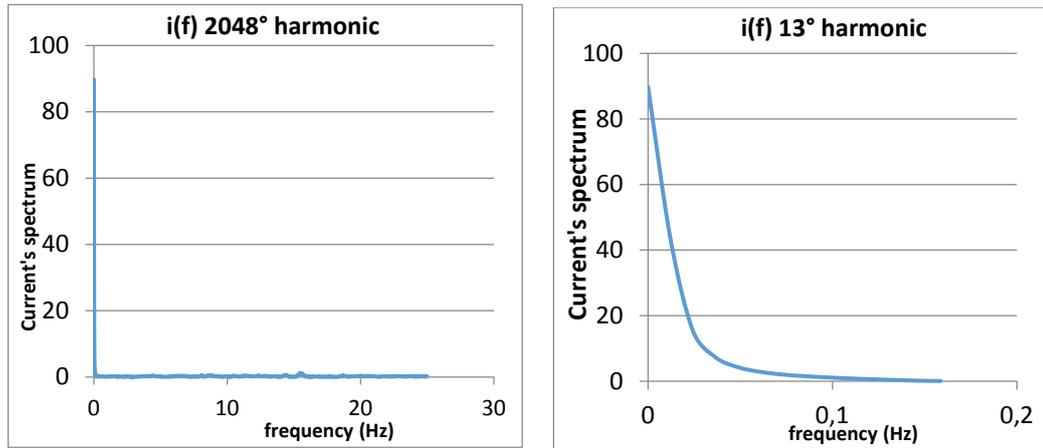
Figure 8.2 - Frequency spectrum of the oscilloscope sampling current
