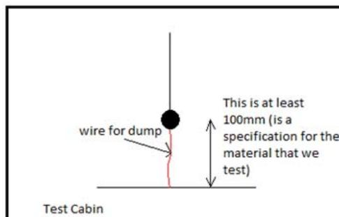
Figure 4.15 - Picture of the test cabin with the wire for the dump
