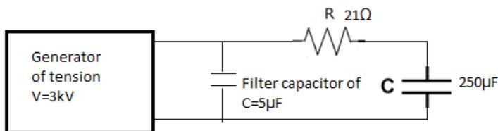
Figure 5.19 - Scheme of a possible filter for the capacitor's charging
