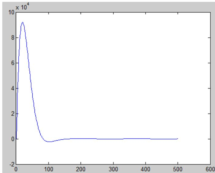
Figure 5.8 - Matlab's simulation of the shape of  $i(t)$  generated at the end of the D-bank's circuit (Current "A" on vertical axis, time " $\mu$ s" on horizontal axis)
