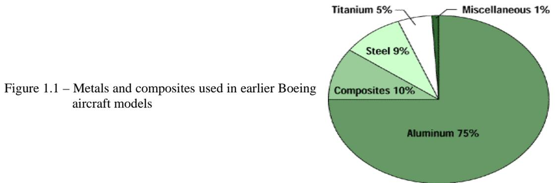
Figure 1.1 – Metals and composites used in earlier Boeing aircraft models
