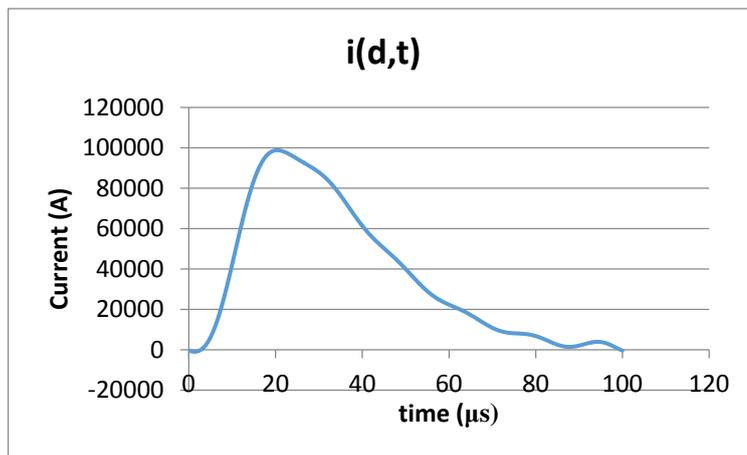
Figure 7.11 –  $i(d, t)$  Current’s shape by plotting in excel the equation 7.8 for the distance of the cable  $d=3,8 \text{ m}$
