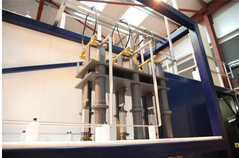
Figure 4.8 - Switch for charging/discharging of the C/D-bank
