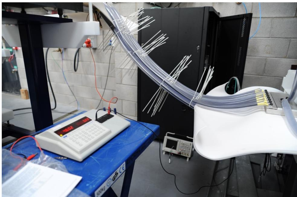
Figure 6.12 - Picture of the eight wires coming inside the test cabin
