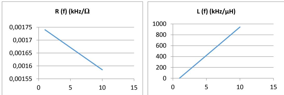
Figure 6.22 – Graphic representation of resistance's and inductance's values in function of the current's frequency applied to the power line (whole extension of the cables)
