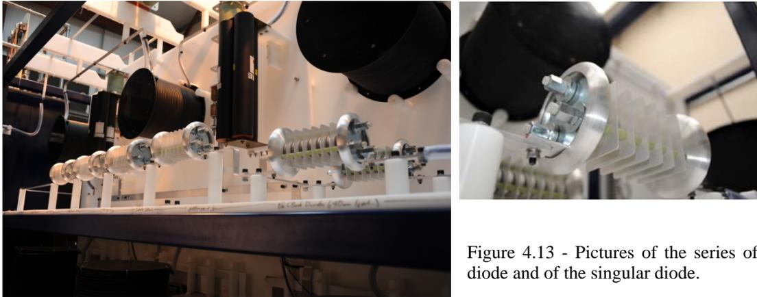
Figure 4.13 - Pictures of the series of diode and of the singular diode.
