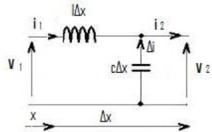
Figure 7.10 – Representation of a generic power line element
