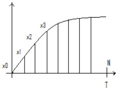
Figure 7.4 - Trapezoidal division (with equal bases of each trapezium) of a generic function to derive the FFT
