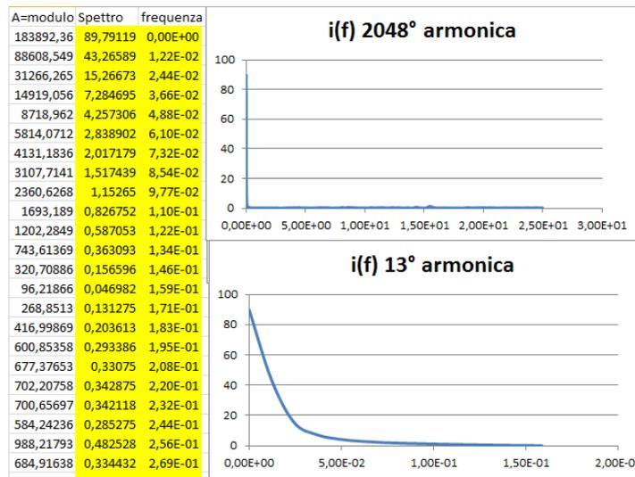
Figure 8.1 – Excel work paper for the harmonic analysis (FFT) of the oscilloscope sampling current's values
