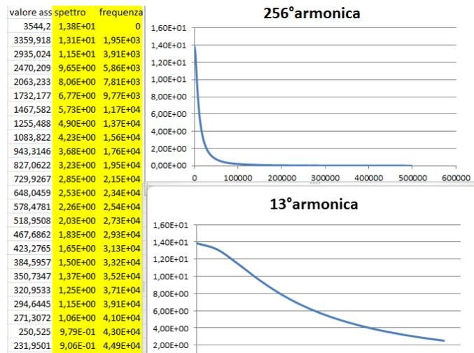
Figure 8.2 - Excel work paper for the harmonic analysis (FFT) of the current's values, taken by the ATP simulation
