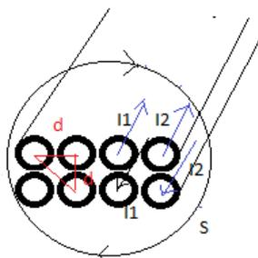
Figure 6.20 - Ampere Low apply for the eight wires
