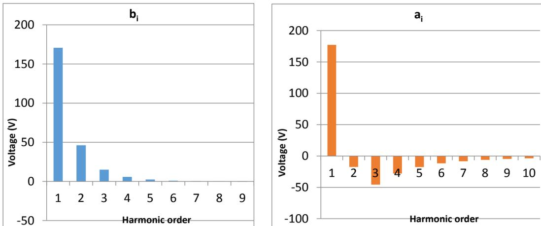
Figure 7.8 - Harmonics tension's values' diagram for the "a<sub>i</sub>" and for the "b<sub>i</sub>" (FFT terms) with a jump of 10 harmonics each step
