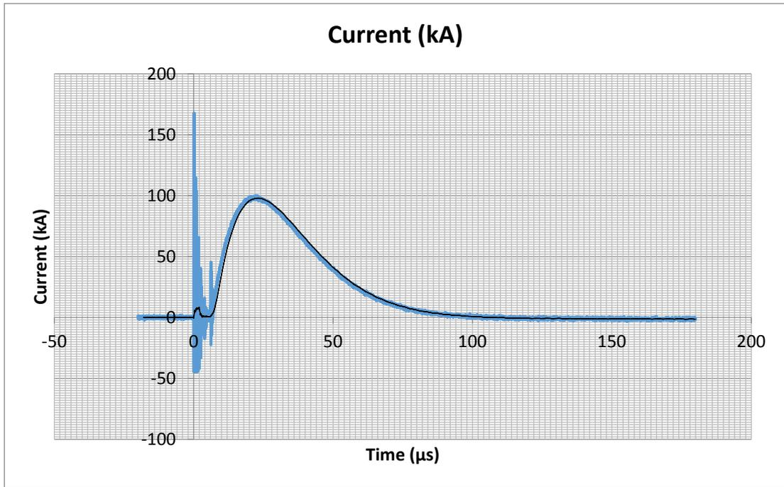
Figure 5.9 –  $i(t)$ -Current's shape obtained by plotting, in excel, the sampling values measured by the oscilloscope during the test of aluminum plate with D-bank's circuit.
