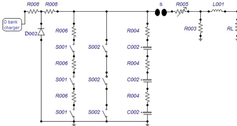
Figure 6.9 - D-bank electric scheme with evidence of the fundamental dissipative component
