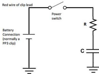
Figure 5.13 - Scheme of the capacitor's charging circuit
