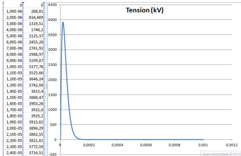
Figure 7.3 – Shape of tension at the end of the D-bank’s circuit by the sampling in excel of the ATP plot’s values
