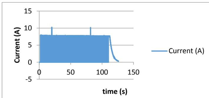
Figure 5.21 - Shape of current (in 6 of the 13 capacitors) during the charging of the C-Bank with the capacitor filter (oscilloscope sampling)
