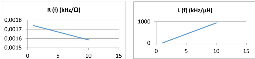
Figure 6.28 – Graphic representation of Resistance's and inductance's values in function of the current's frequency applied to the power line (cables of coming back, outside the test cabin)
