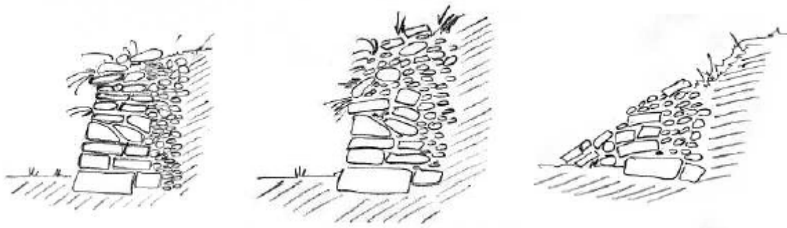
Figure 1.11. a) Localized degradation of wall top; b) Widespread degradation; c) Wall portion collapse (figures from Sangiorgi et al., 2006).
