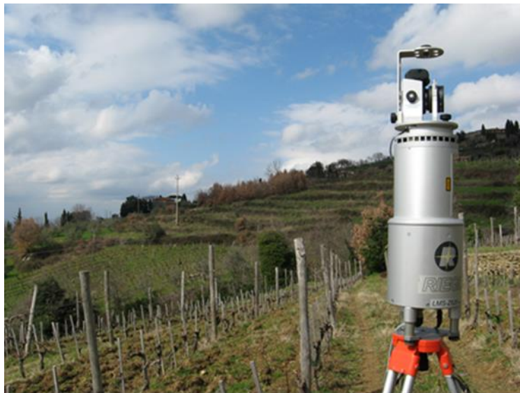
Figure 6.5. Terrestrial Laser Scanner Riegl LMS-Z620 with camera, used in Lamole site (picture by S. Calligaro).
