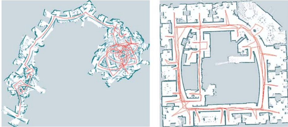
Figure 1.3: Occupancy grid map generated from laser range data, based on pure odometry (left) and resulting from a scan-matching particle filter algorithm (right) [7].
