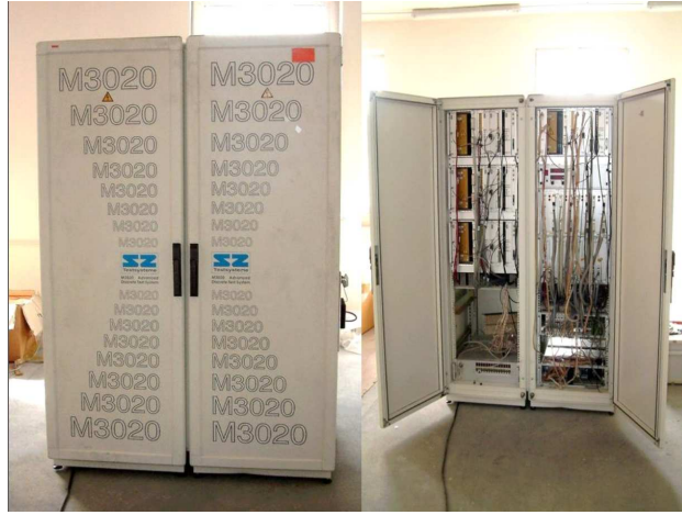
Figure 4.9: Static Tester M3020 used for measuring the static R_{dson} .
