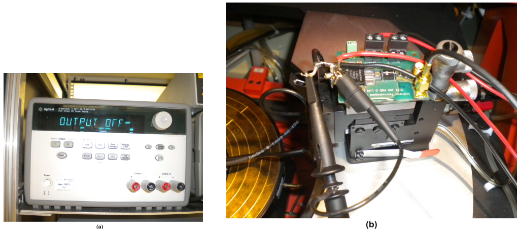
Figure 5.15: GaN DReaM Setup; Agilent E3649A auxiliary Power Supply, used in the gate driving of the DUT (a), Gate Driver mounted on PCB on the gate manipulator inside the wafer station (b).
