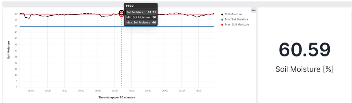
Figure 8.46: Soil moisture graph out of range
