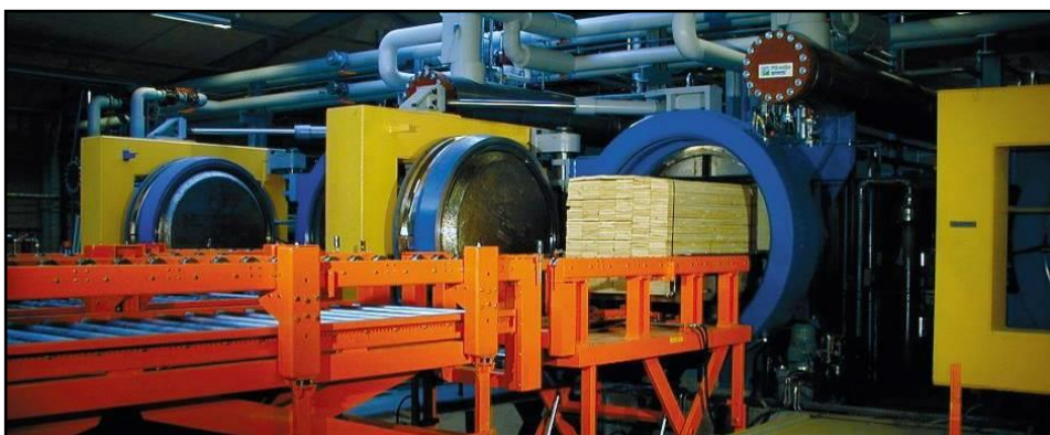
Figure 5.2. Automatic charging of the wood in the impregnation vessel. The 3 vessels can be seen. [41]
