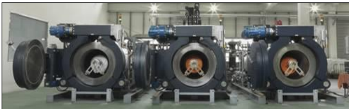
Figure 5.3. Impregnation vessels of the supercritical dyeing plant [39]
