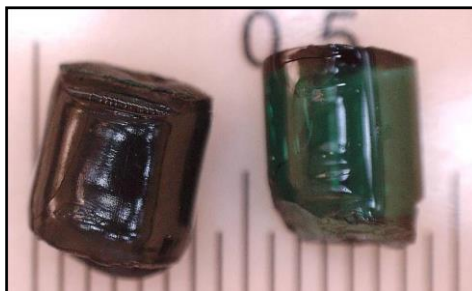
Figure 3.8. Opaque semicrystalline pellet (on the left), amorphous pellet (on the right).
