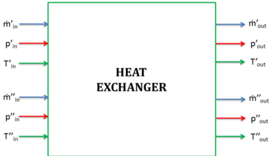
Figure 3.19 Input output diagram of dynamic model for heat exchangers.
