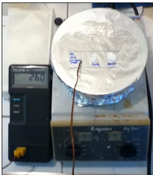
Figure 2.2. Melt test equipment, composed by a hot plate supporting the glass slide with the samples and a digital termocouple iron-costantan.
