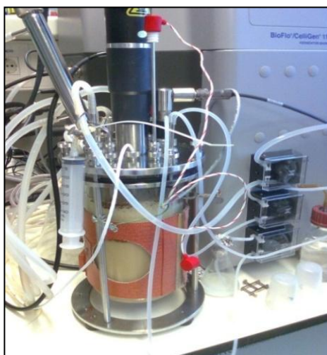
Figure A1. One of the two STR of 2 liters of IBB/CEBQ laboratories in IST Lisbon. Inside, the fermentation broth in which B. sacchari accumulates PHA.
