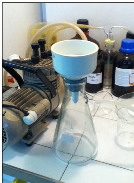
Figure 3.3. Buchner filtration equipment. On the left the vacuum pump.
