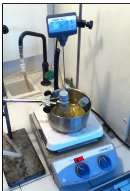
Figure 3.4. Solubility measurement equipment. The temperature on the hot stirred plate is decided and controlled by the digital immersion thermometer
